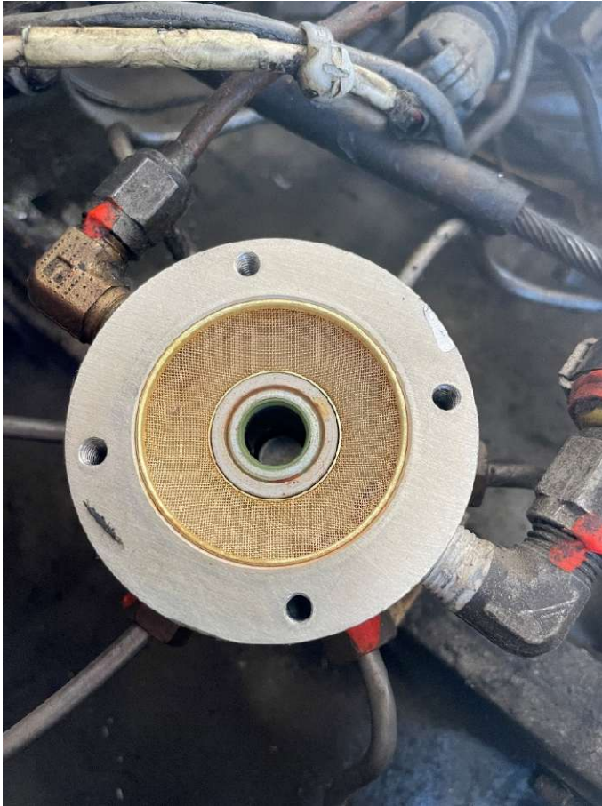
Photo 5: Fuel Screen from Engine Fuel Flow Divider
