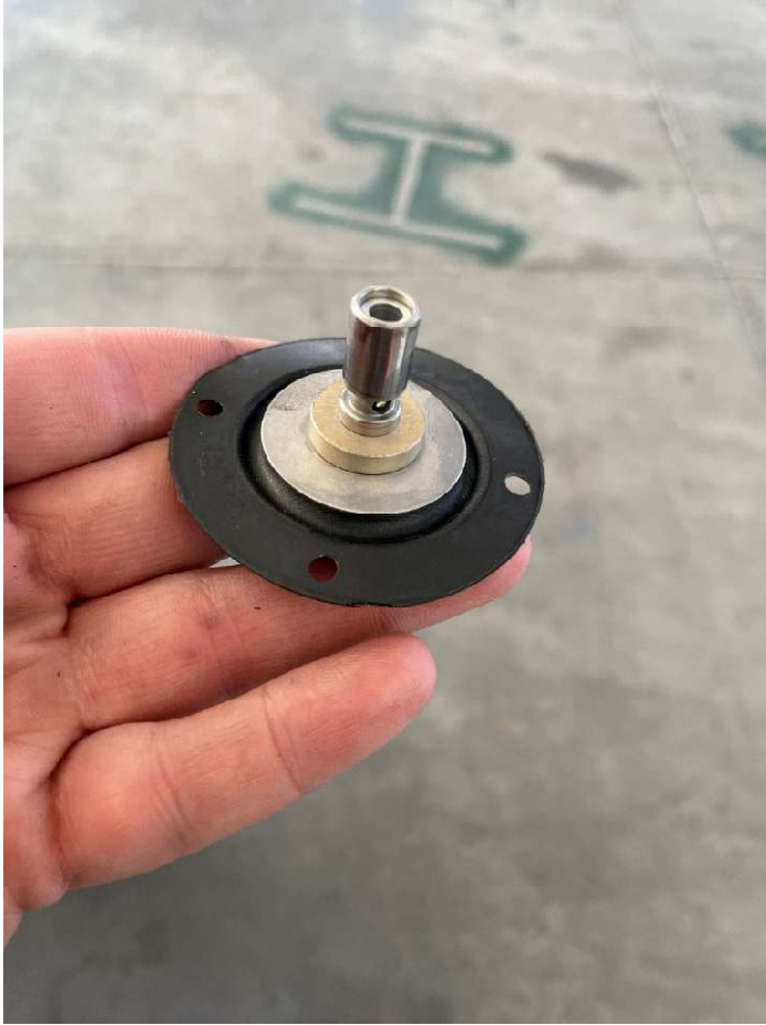
Photo 6: Diaphragm from Fuel Flow Divider
