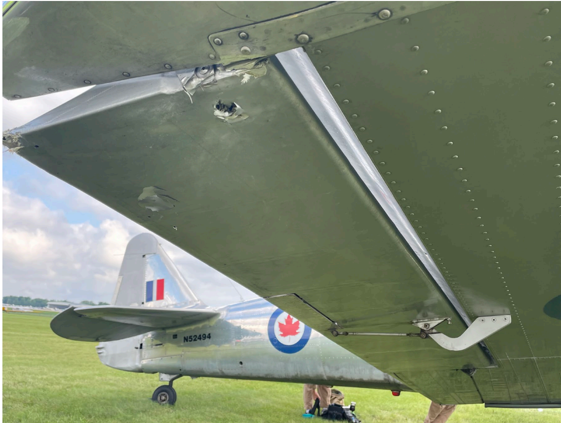
Photograph 2 - View of right aileron damage
