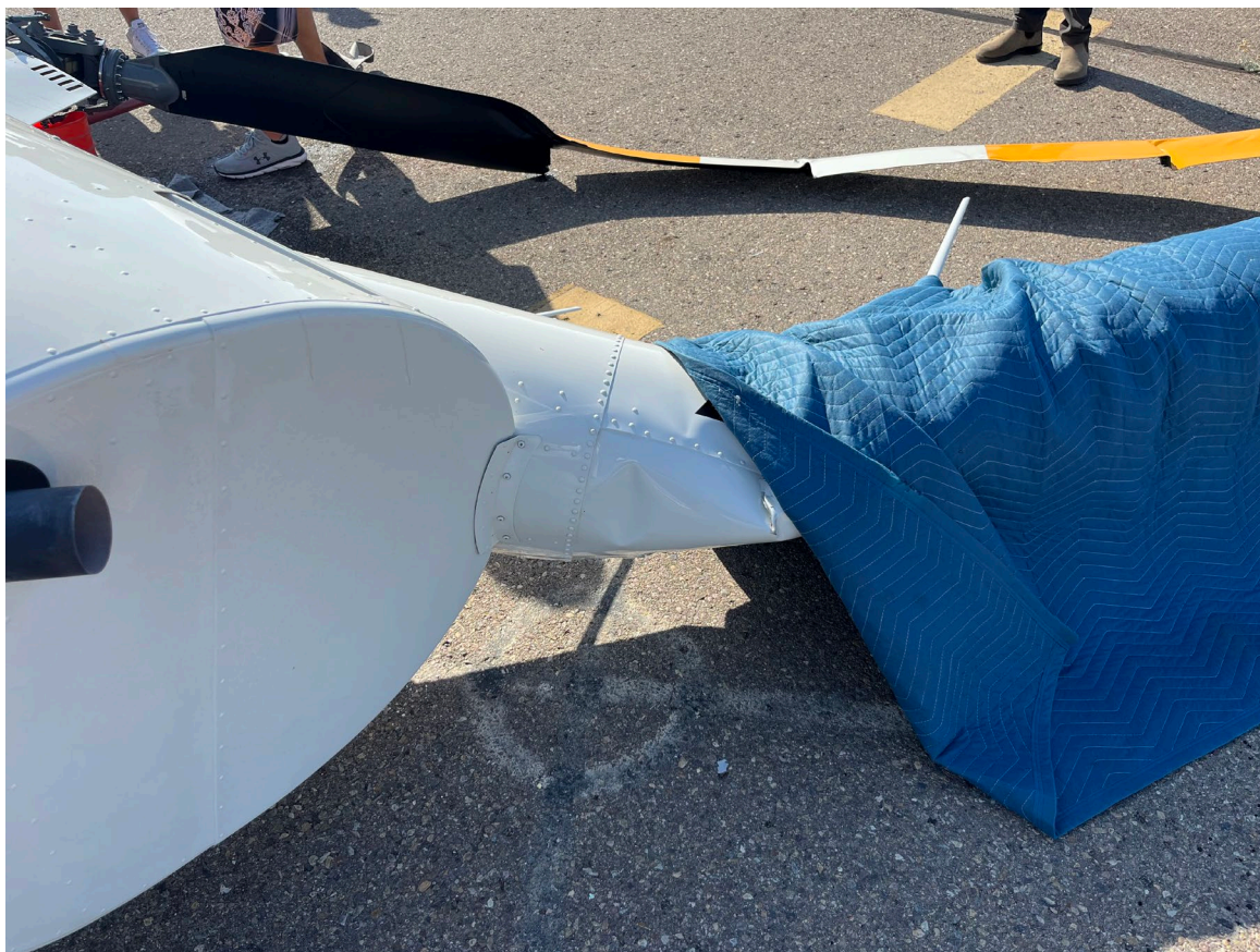
Photograph 3 - View of substantial damage to tailboom. (Courtesy of the FAA.)
