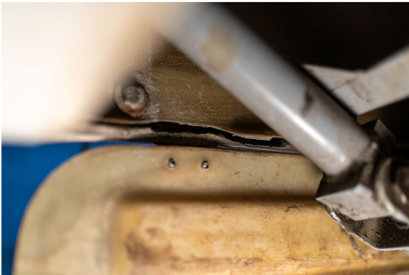
Photo 2 – Gap between wheel well and fuselage (courtesy of pilot/owner)
