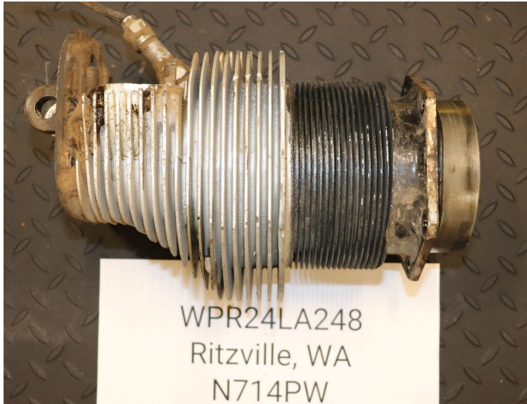
Figure 13: View of the No. 2 cylinder.
