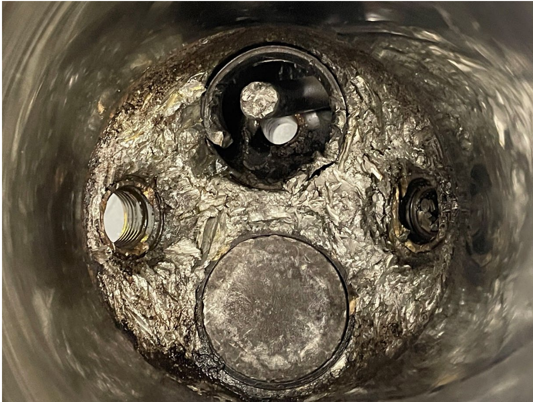
Figure 5: View of No. 2 cylinder combustion dome
