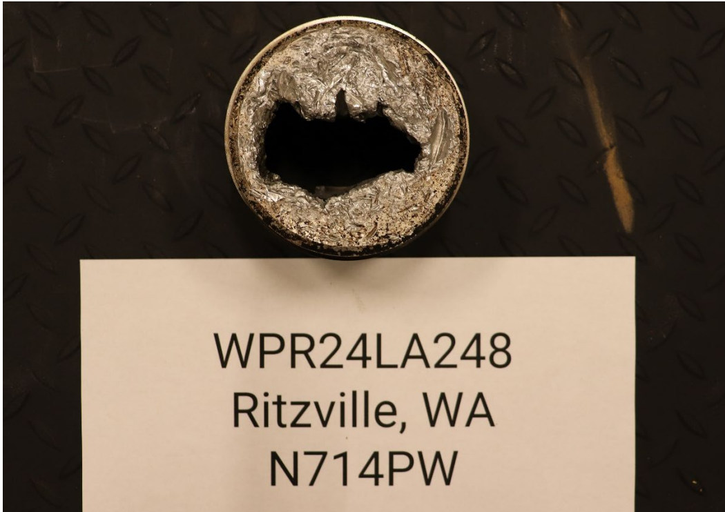
Figure 14: View of No. 2 piston.
