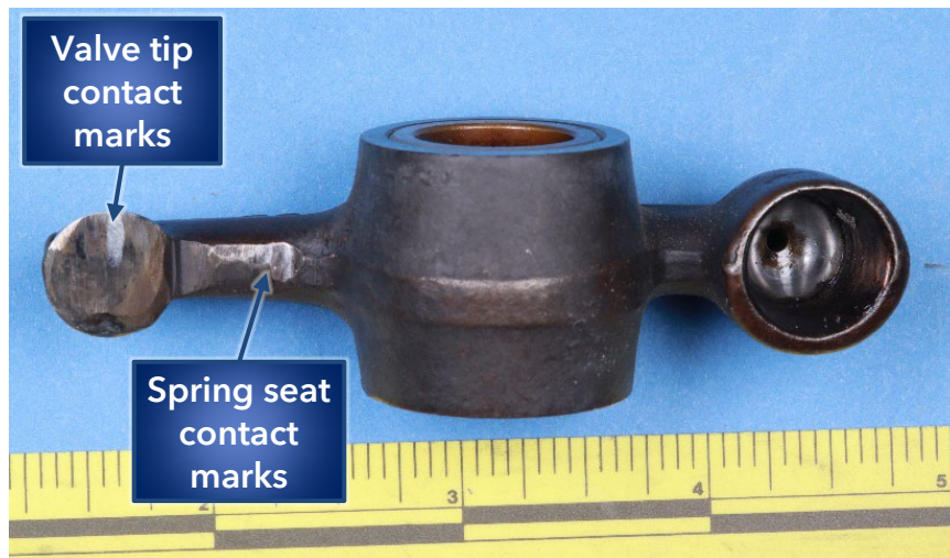
Figure 2. Exhaust rocker arm showing offset contact marks on the rocker pad and seat contact marks on the arm.
