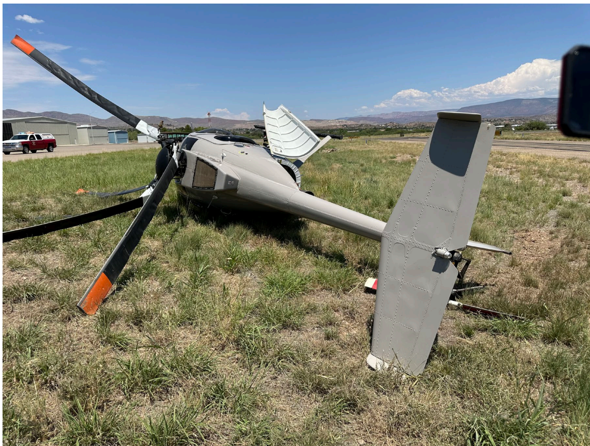
Photograph 1 - View of accident helicopter with view of damage to the main rotor blades (Courtesy of operator)
