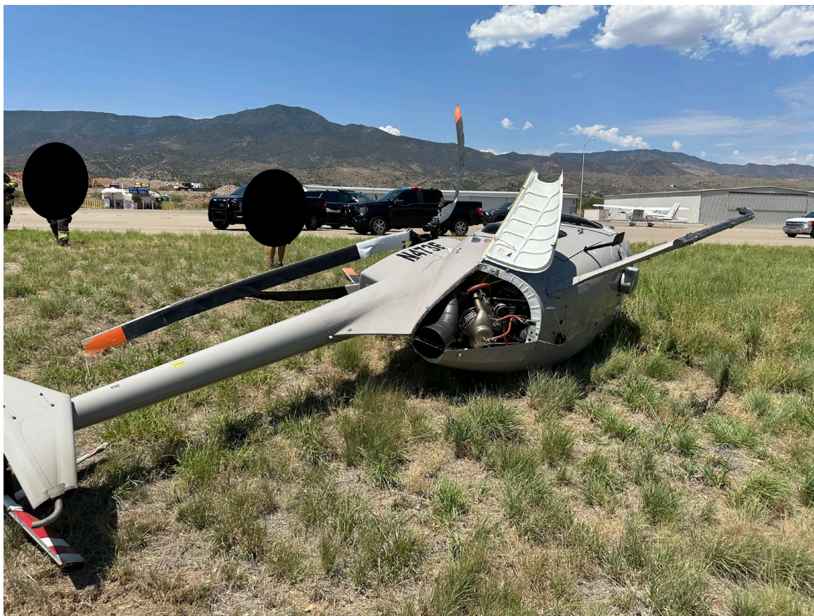
Photograph 2 - View of helicopter laying on its left side, with damage to lower fuselage and missing left skid (Courtesy of operator)
