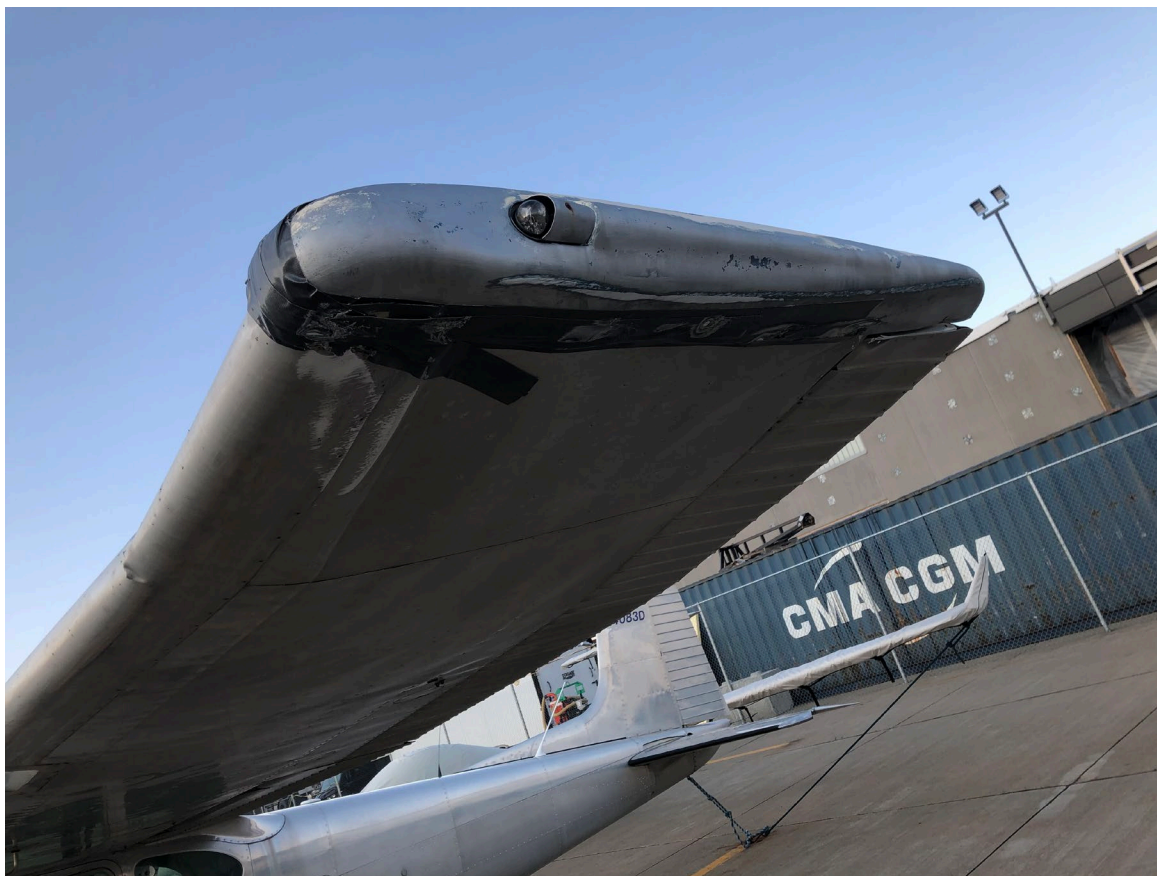
Photograph 2 - View of substantial damage to the left wing. (Courtesy of pilot.)
