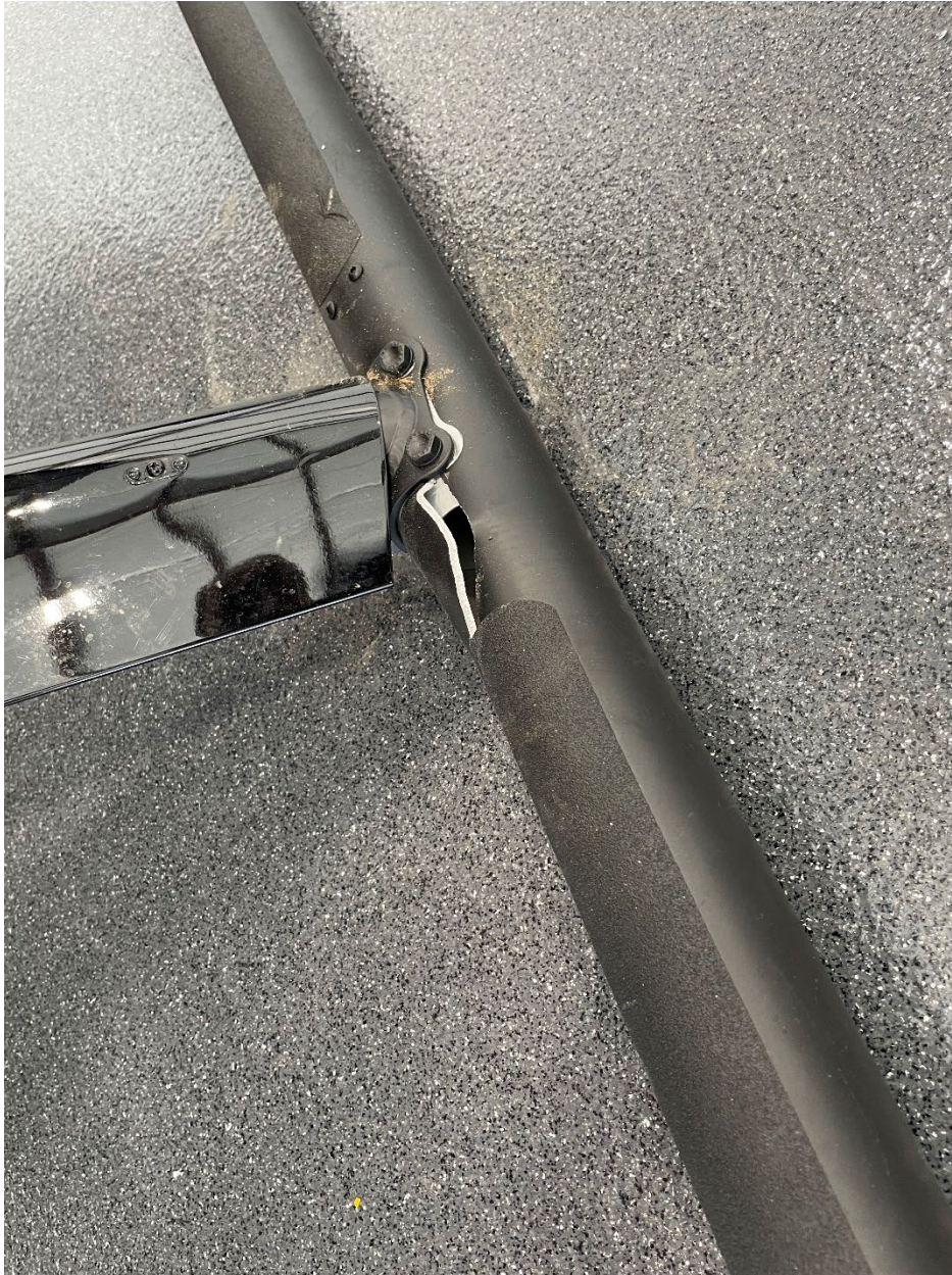
Figure 5. Fracture at the right skid near the forward saddle area.
