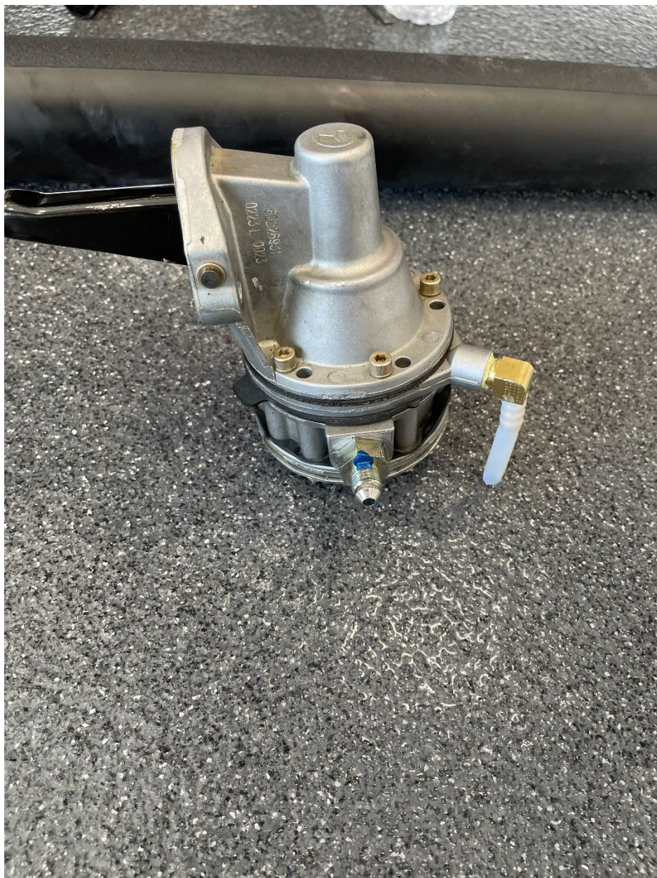
Figure 11. View of removed fuel pump
