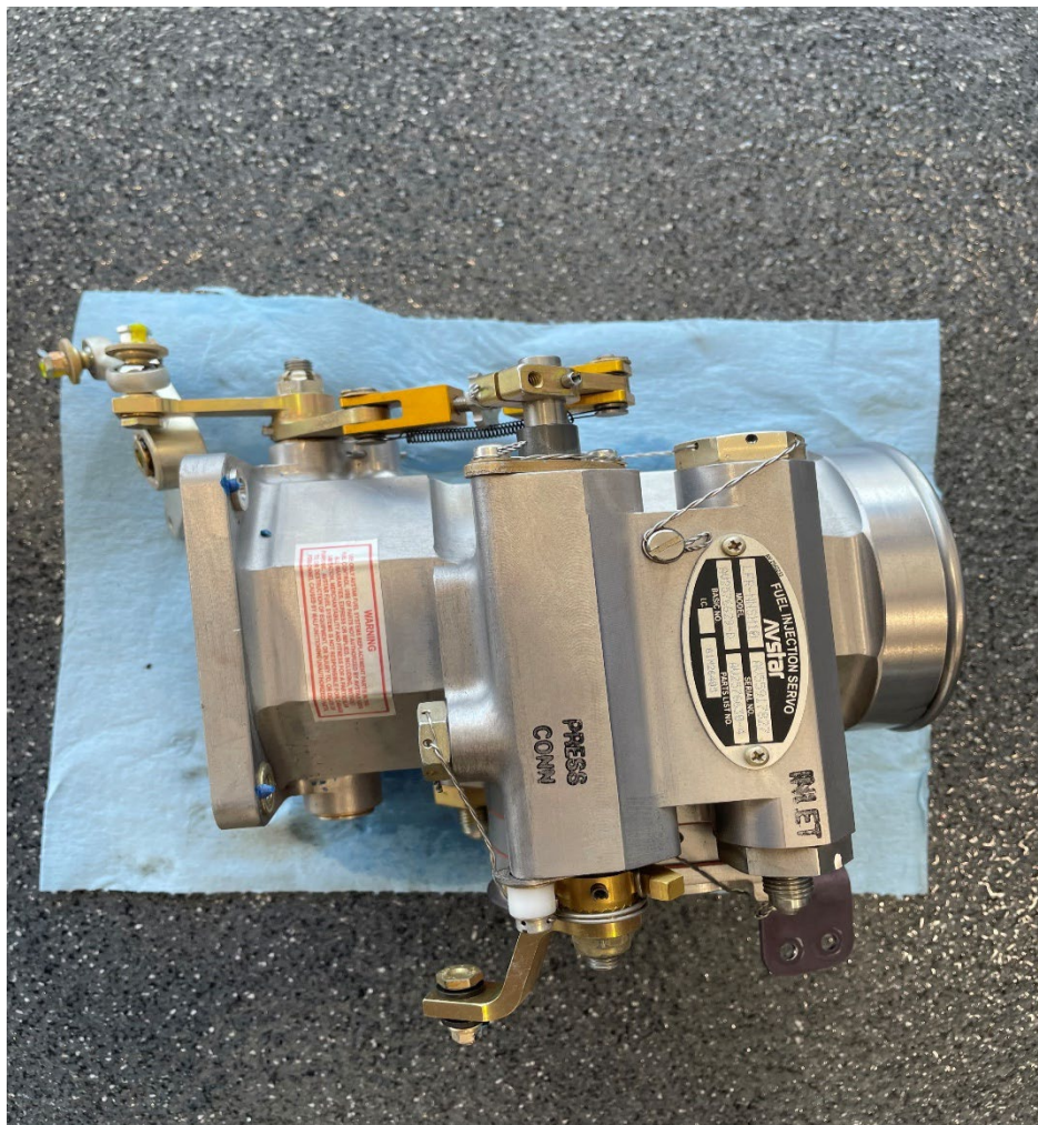
Figure 10. View of removed fuel servo
