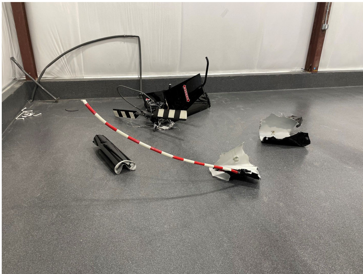
Figure 4. Aft tail cone components, tail rotor gearbox and tail rotor assembly.
