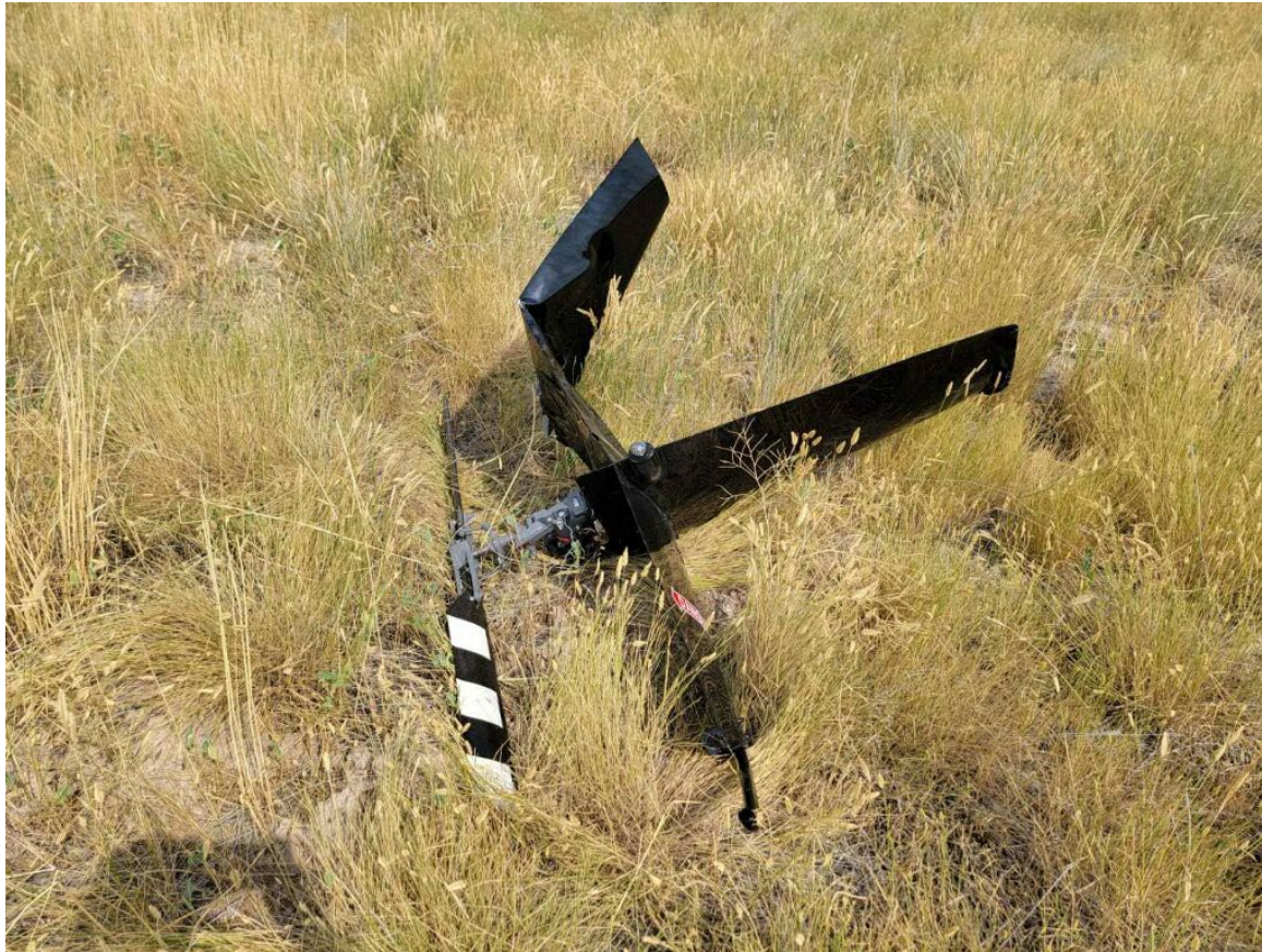
Photograph 2 - View of separated tail rotor assembly and vertical & horizontal stabilizer in an open field (Courtesy of pilot)
