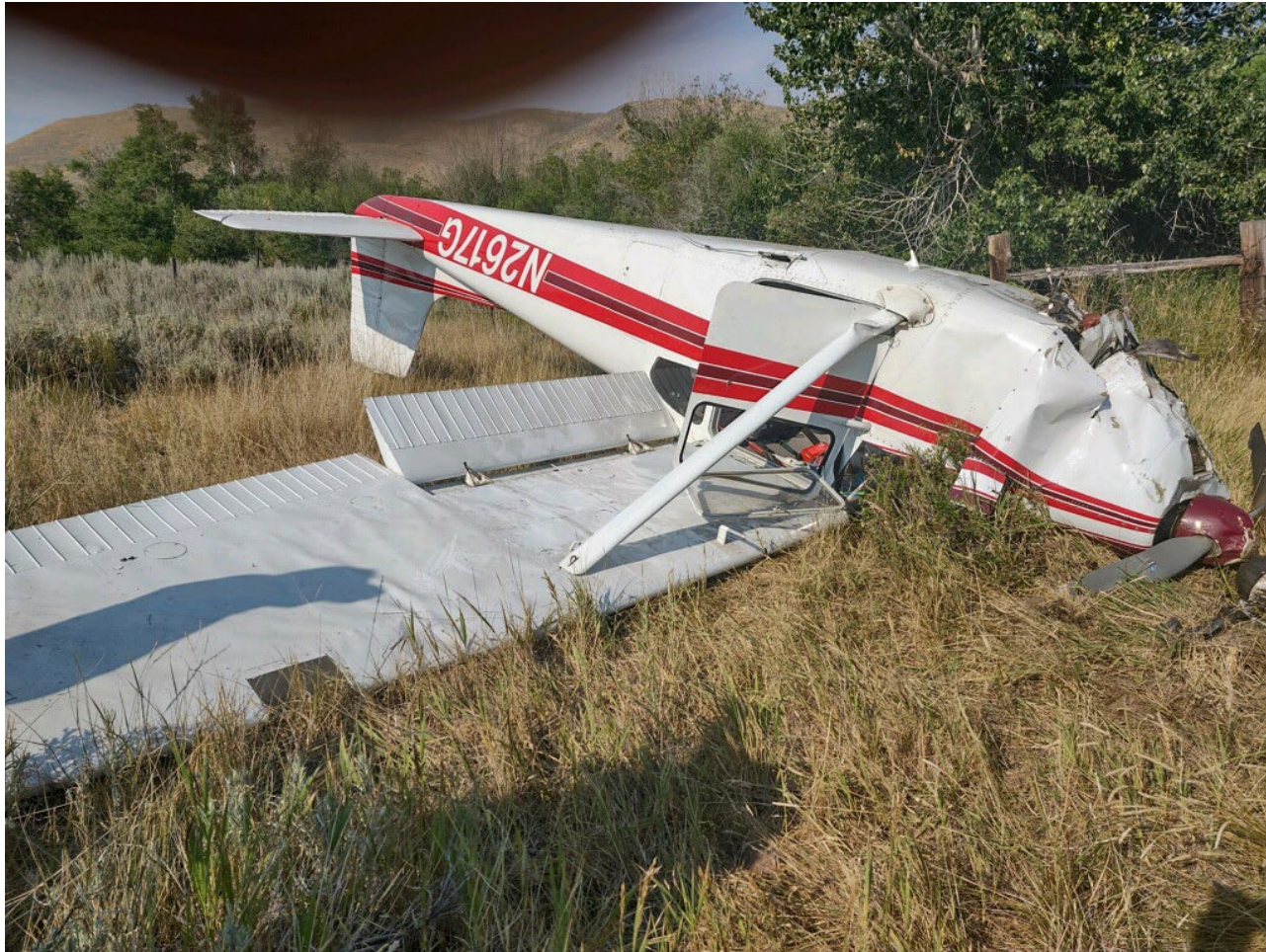
Photograph 1 - View of substantial damage to the left wing lift strut and damage to the horizontal stabilizer (Courtesy of pilot)
