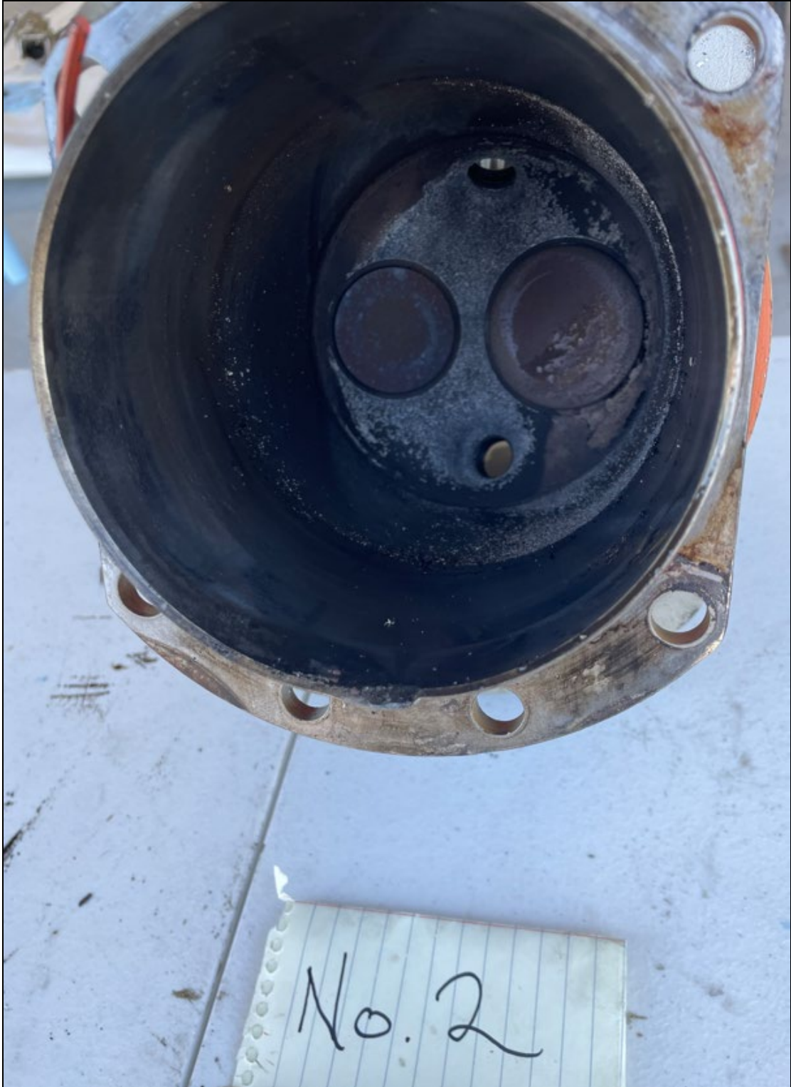
Figure 9: View of No. 2 cylinder barrel, head, exhaust and intake valves
