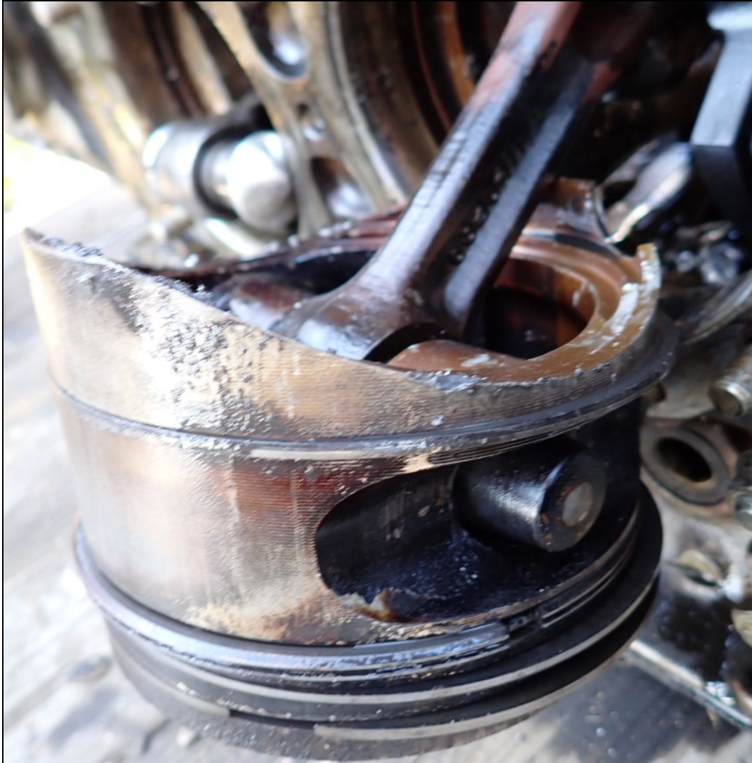
Figure 13: View of No. 3 connecting rod and piston skirt
