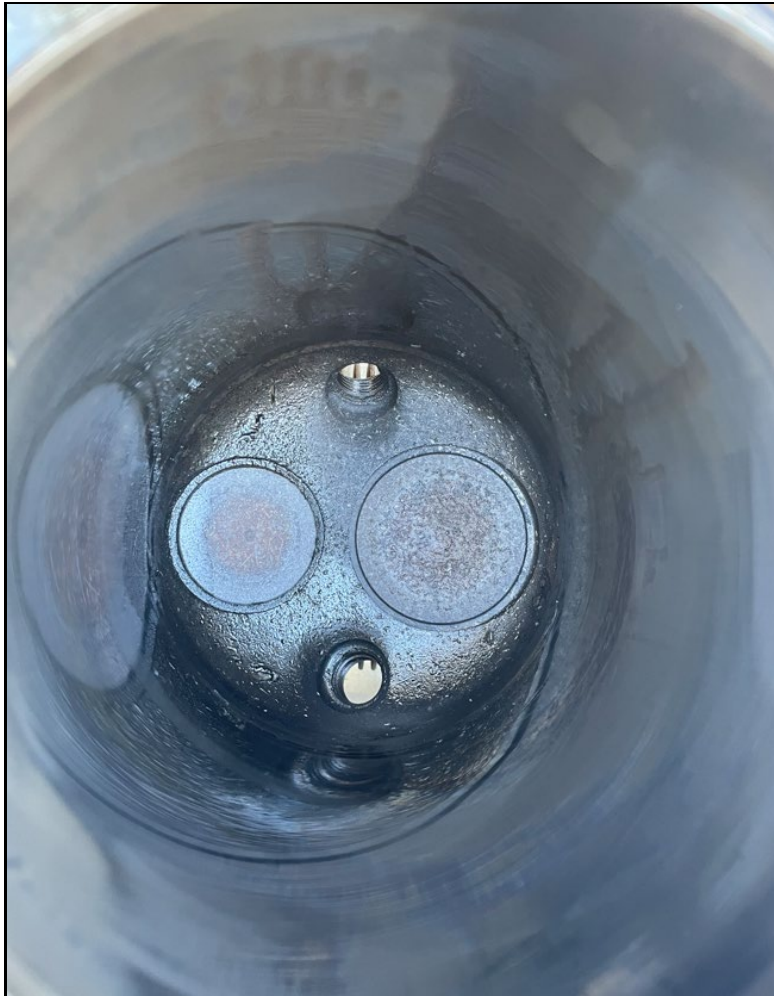
Figure 19: View of No. 5 cylinder walls, head, exhaust and intake valves
