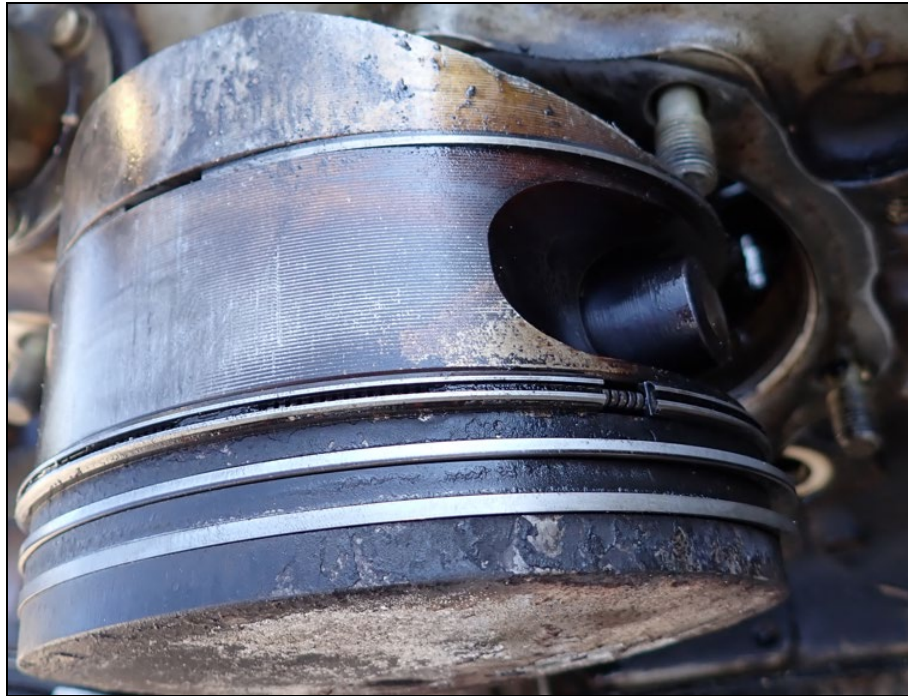
Figure 17: View of No. 4 piston skirt
