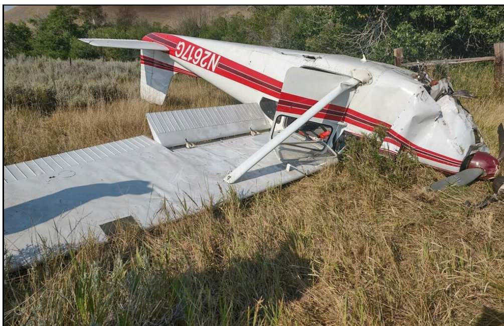
Figure 1: View of inverted accident airplane at the accident site
