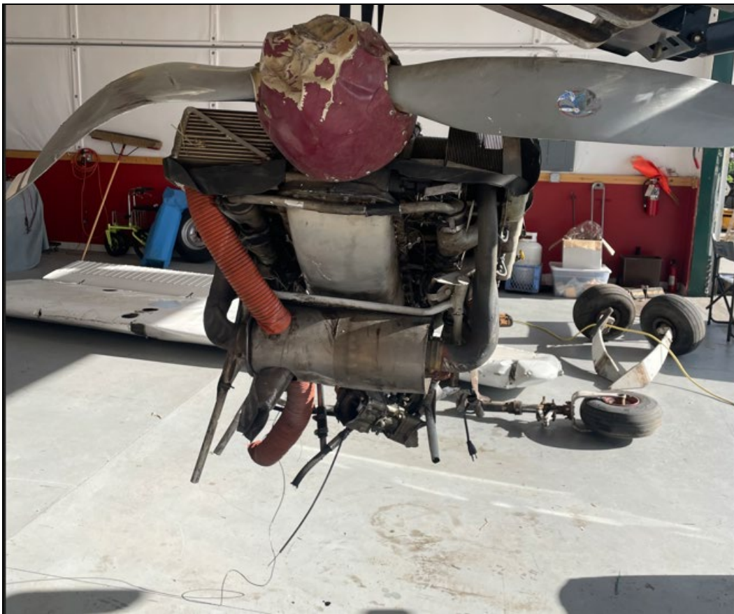
Figure 2: View of the accident engine separated from the airframe
