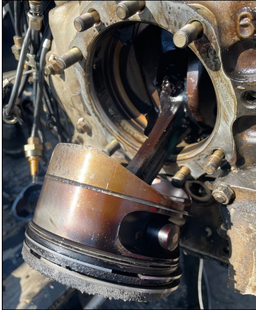
Figure 23: View of No. 6 piston and connecting rod
