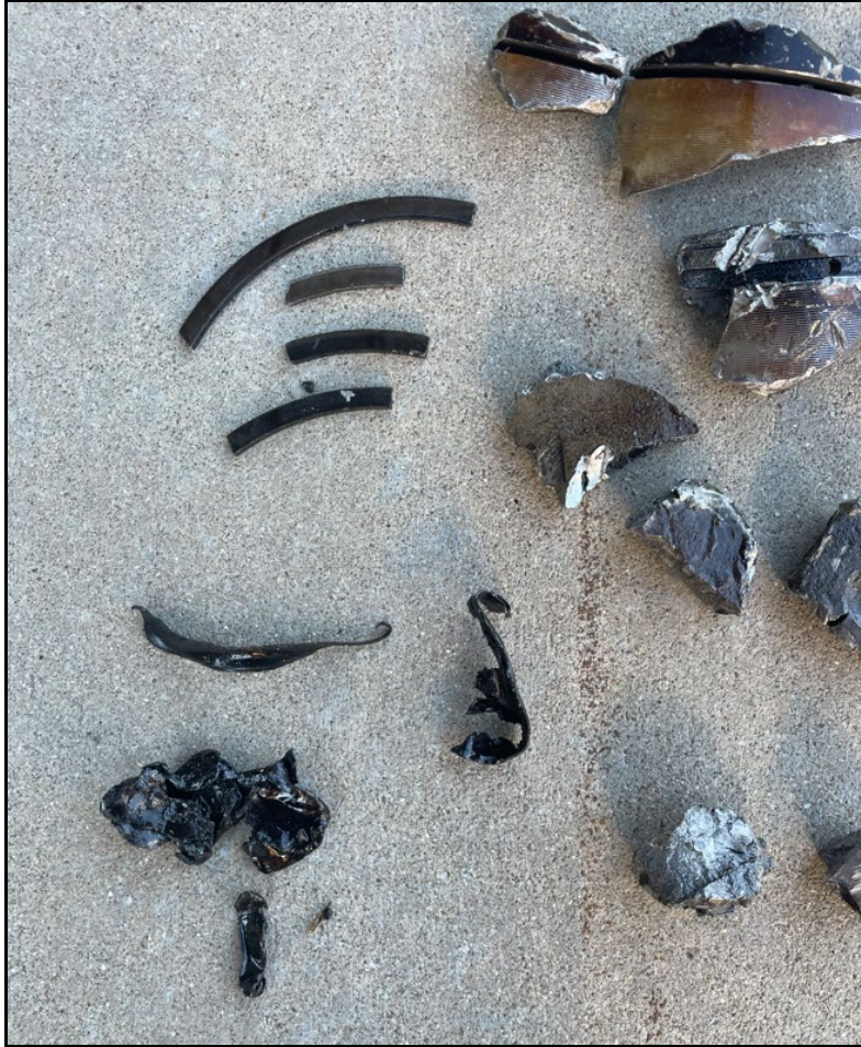
Figure 4: View of the piston and cylinder material found in the engine oil sump
