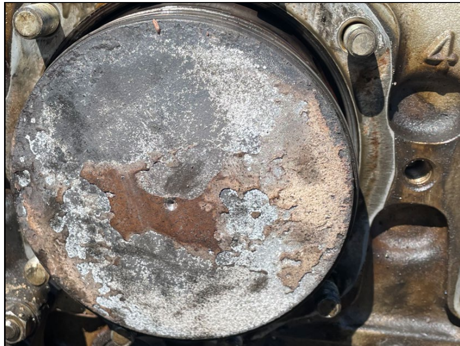
Figure 18: View of No. 4 piston crown
