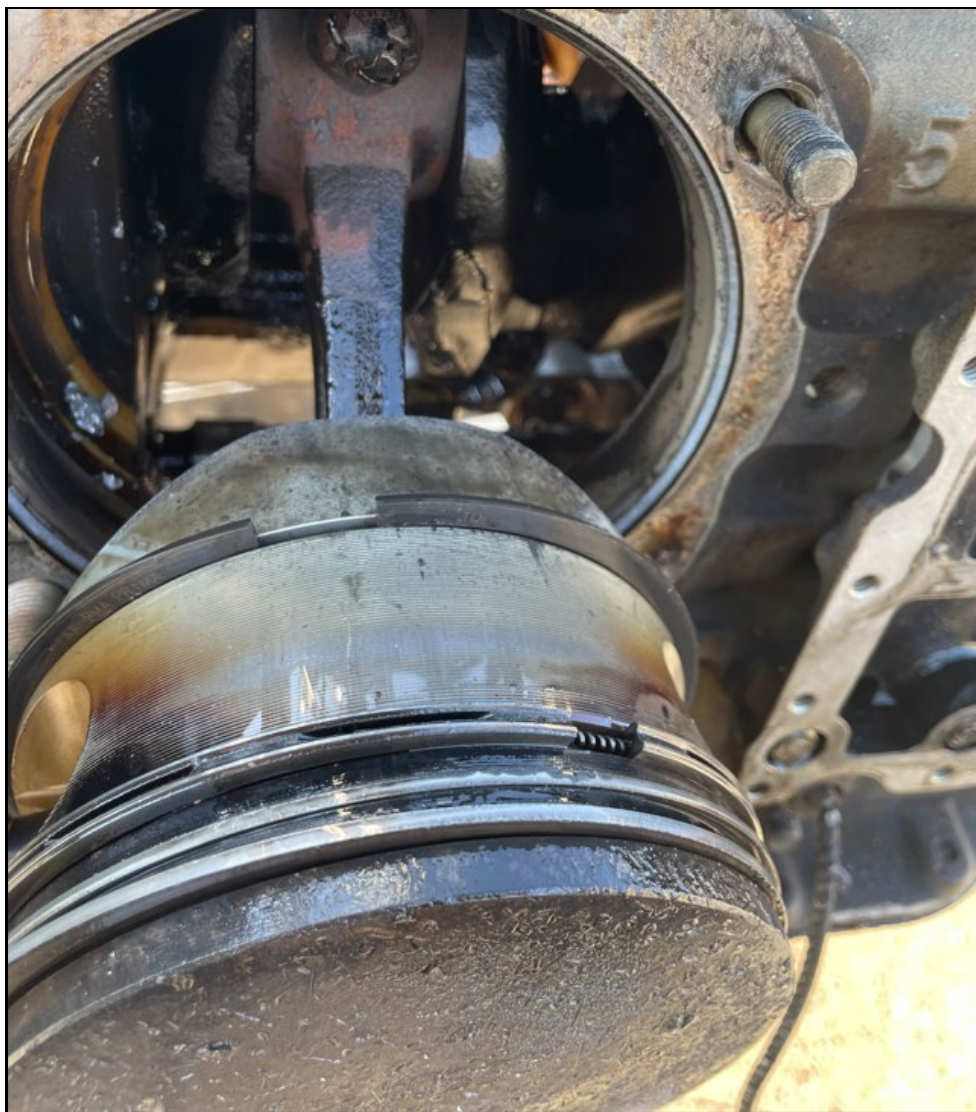
Figure 20: View of No. 5 piston and connecting rod
