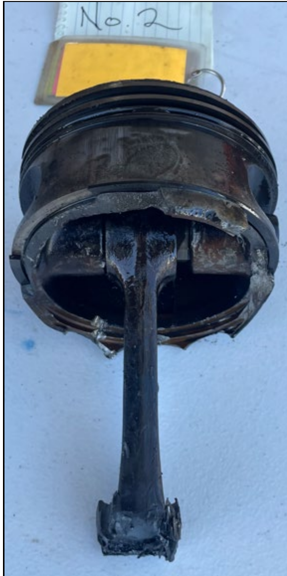
Figure 9: View of No. 2 connecting rod failure and piston skirt damage
