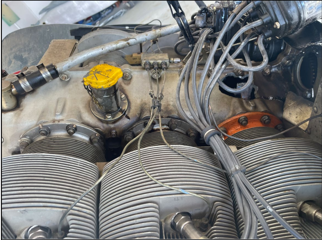
Figure 3: View of hole in the crankcase above the No. 2 cylinder, and right separated magneto
