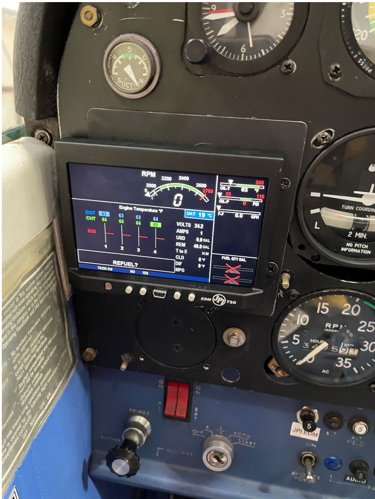
Figure 7. Exemplar electrical system with accident voltage regulator showing 24.2 volts.
