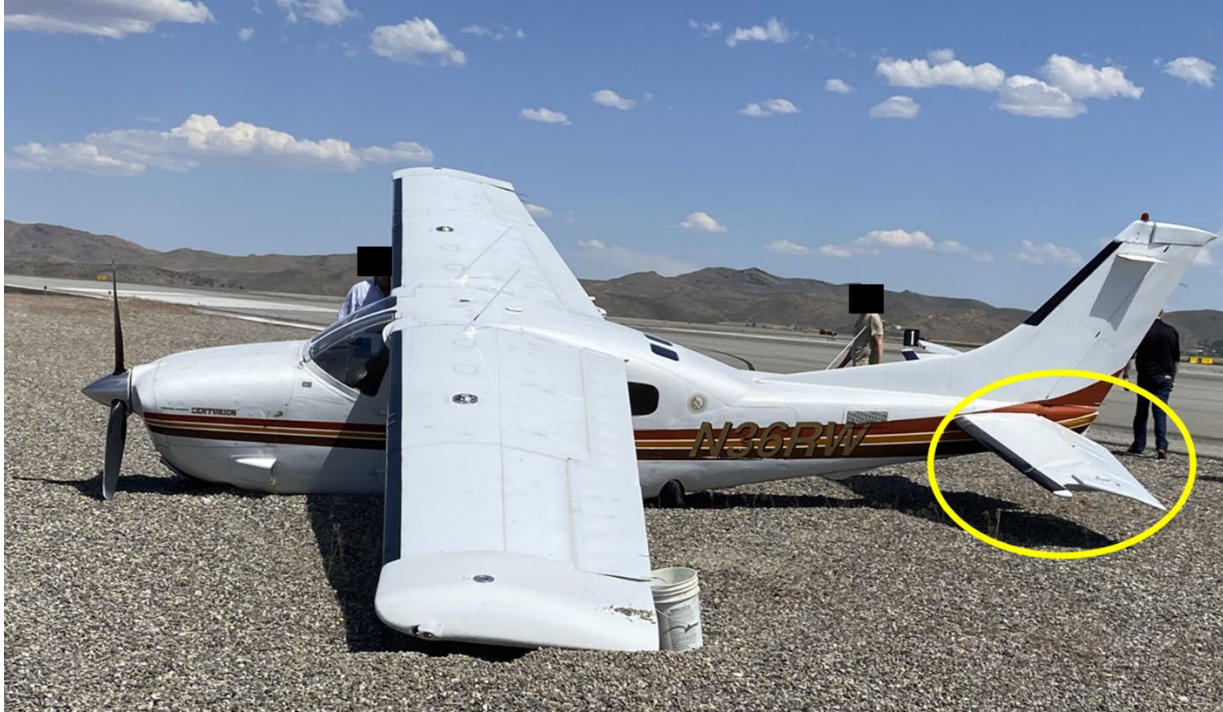
Figure 1. Photo of N36RW showing substantial damage to the left horizontal stabilizer and elevator (Photo courtesy of the pilot).
