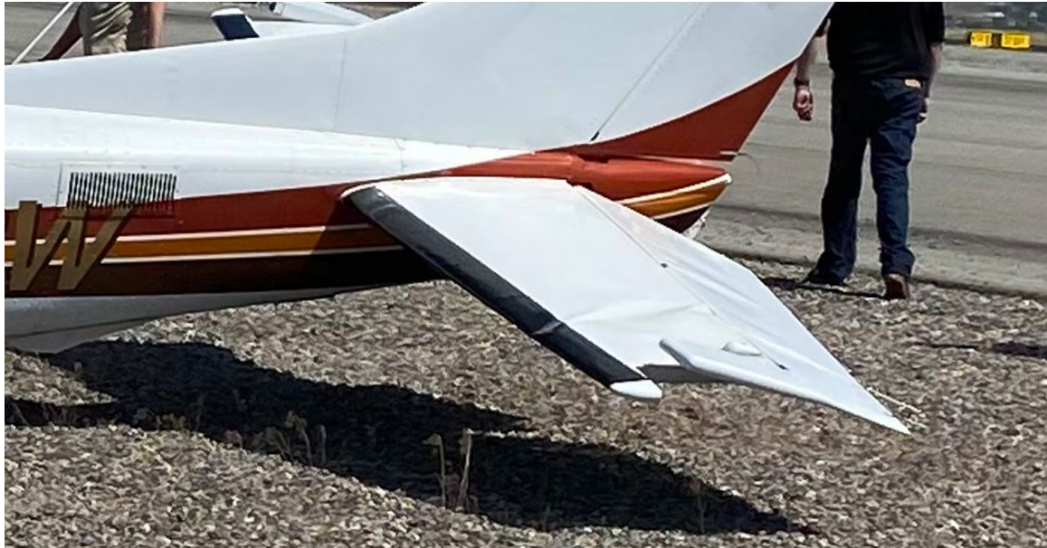
Photograph 3 - Substantial damage to left horizontal stabilizer and elevator. (Courtesy of pilot)
