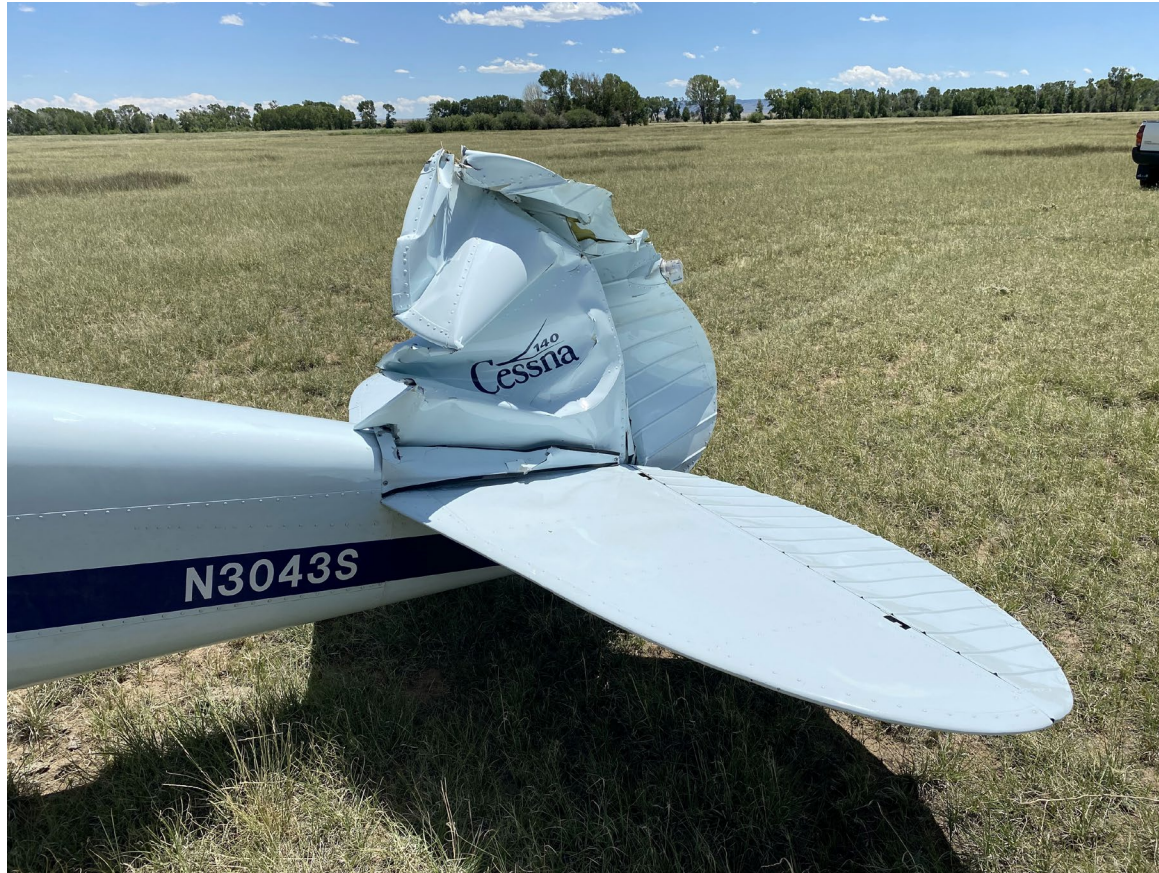
Photograph 3 - View of substantial damage to empennage. (Courtesy of pilot.)
