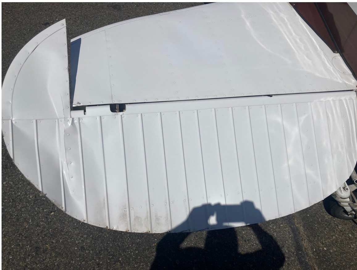
Photograph 2 - Left elevator damage (Courtesy of pilot)
