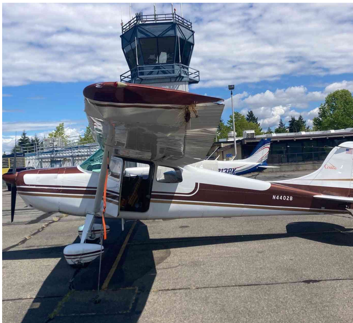
Photograph 1 - Wing damage (Courtesy of pilot)
