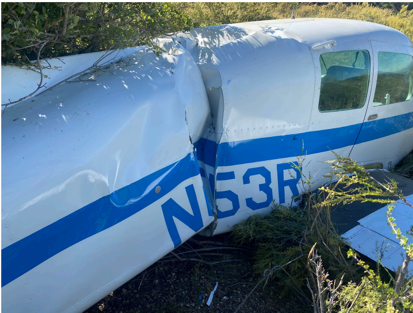
Photograph 2 - View of substantial damage to aft fuselage. (Courtesy of Sheriff's Department.)
