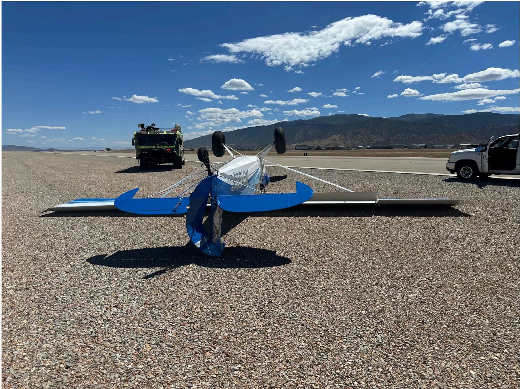
Photo 1 – View of damage to vertical stabilizer, rudder, and right wing lift strut. (Courtesy airport ops)
