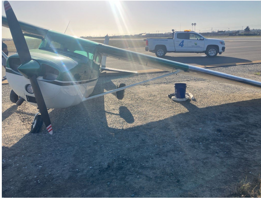
Photograph 1 - View of airplane resting on its left wing, left horizontal stabilizer, and left elevator (Courtesy of Student Pilot)
