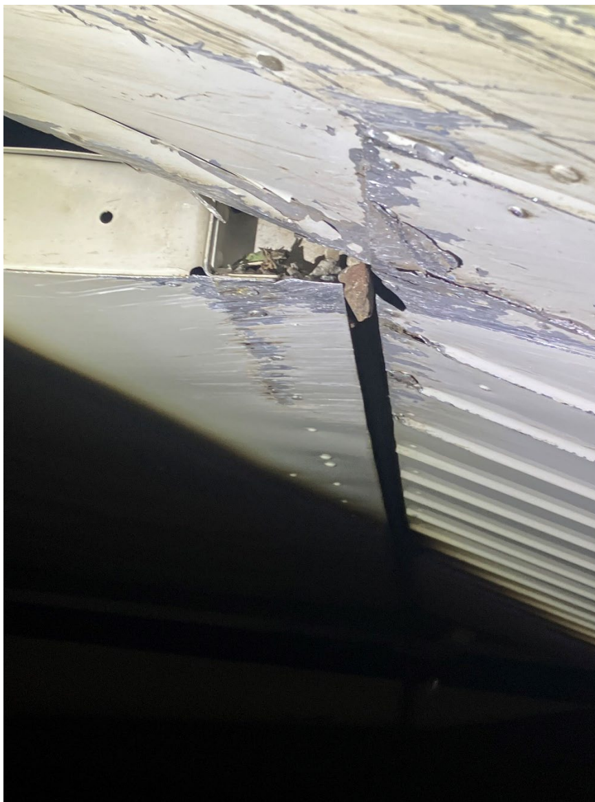
Photograph 2 - View of damage to horizontal stabilizer and elevator (Courtesy of Student Pilot)
