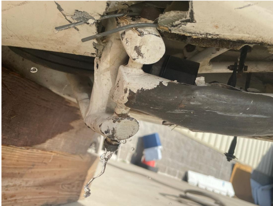
Photograph 6: View of water leak from fuel tank, nose landing gear
