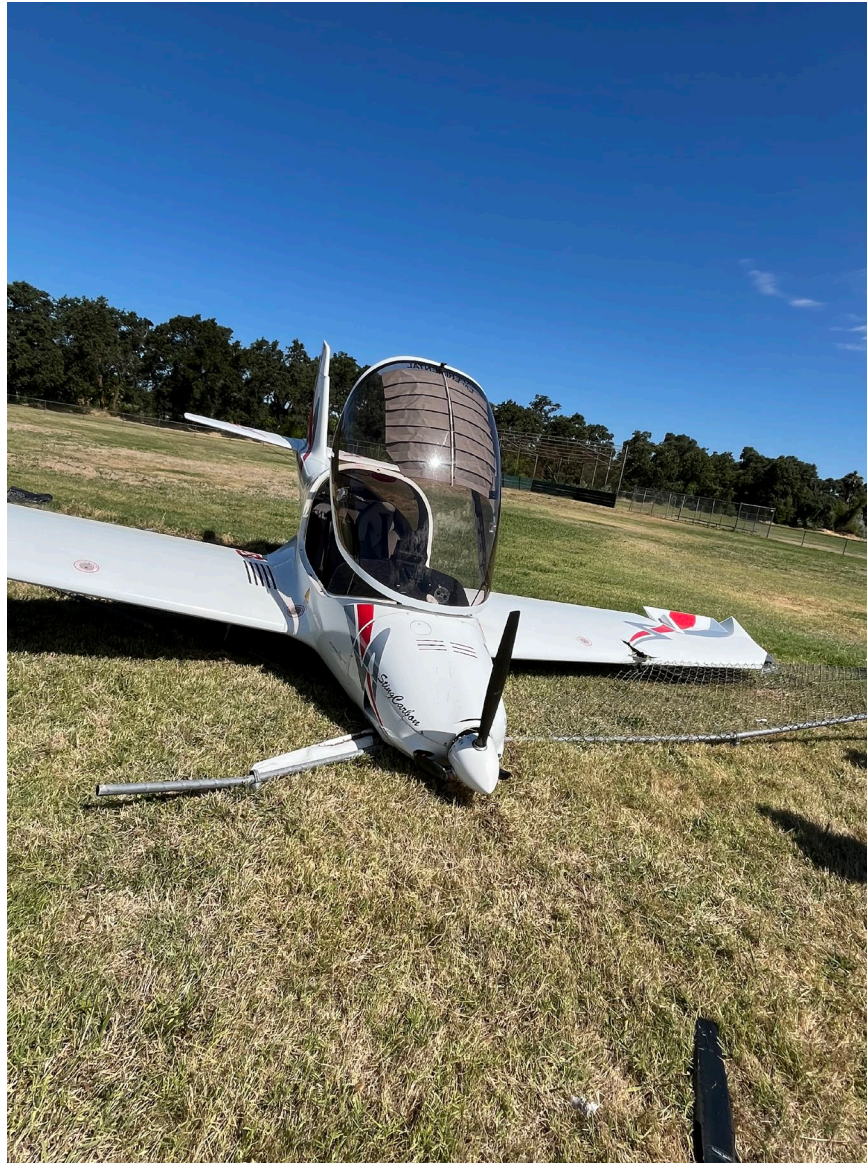
Photograph 2 - Front View of Airplane with Damaged Left Wing (Courtesy of Law Enforcement)
