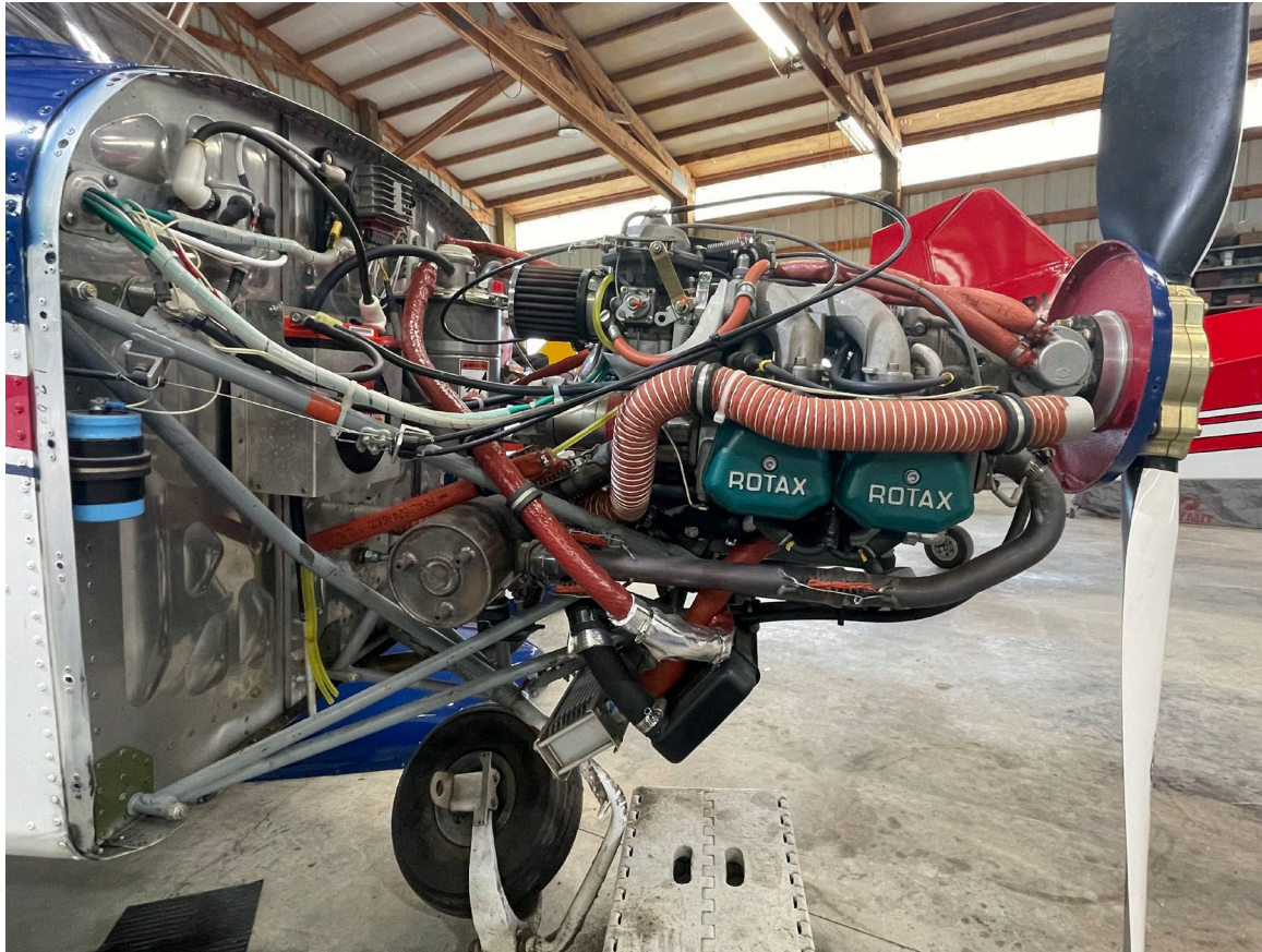
Photograph 3 - View of substantial damage to engine mount. (Courtesy of FAA.)
