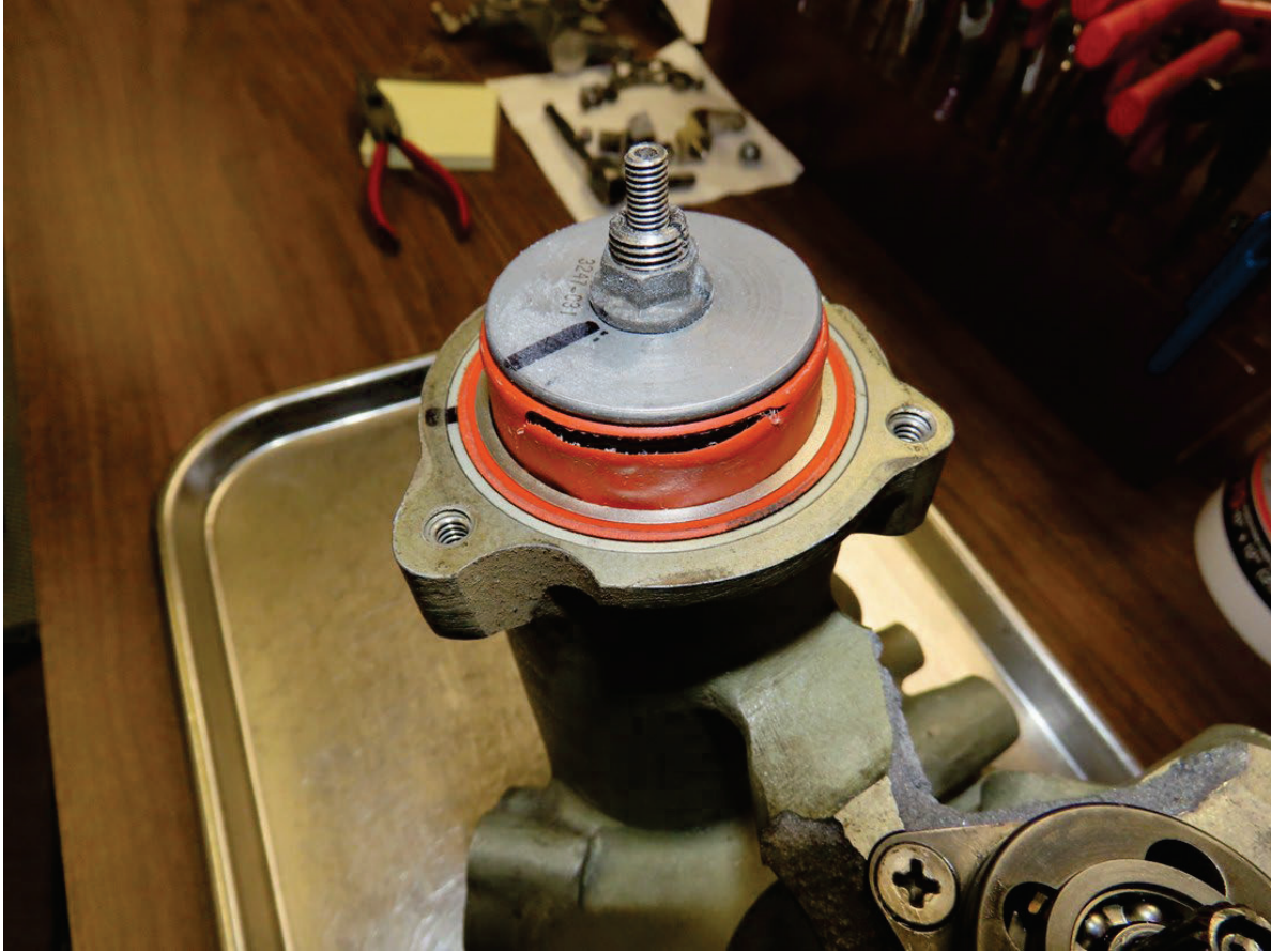
Figure 6- Ps3 Diaphragm Tear
