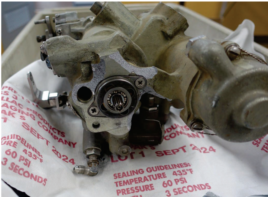
Figure 4- FCU Mounting Flange Damage
