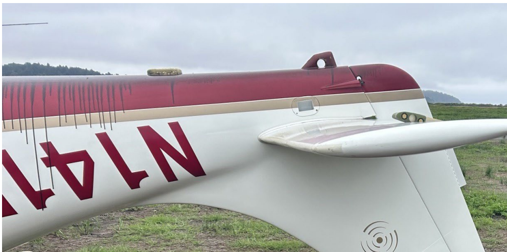
Figure 2 - Oil on belly of airplane at the tail (photo courtesy of the pilot)
