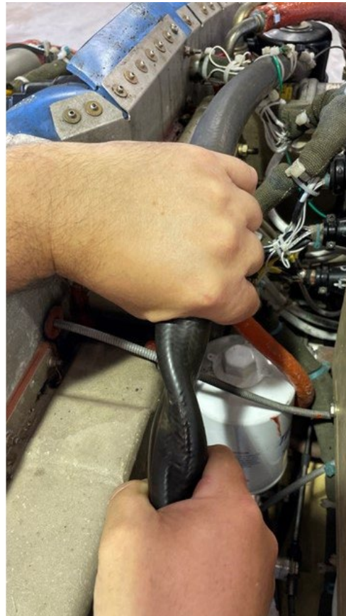
Figure 4 - Oil breather tube with kink circled on left and twisted closed on right.
