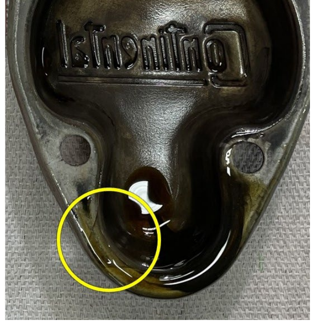
Figure 6 - Witness mark of misaligned gasket.
