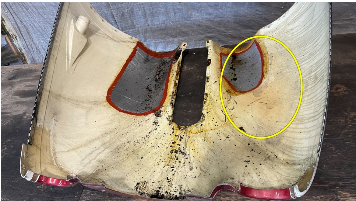
Figure 7 - Oil predominantly in lower left of cowling adjacent to cylinder 2.
