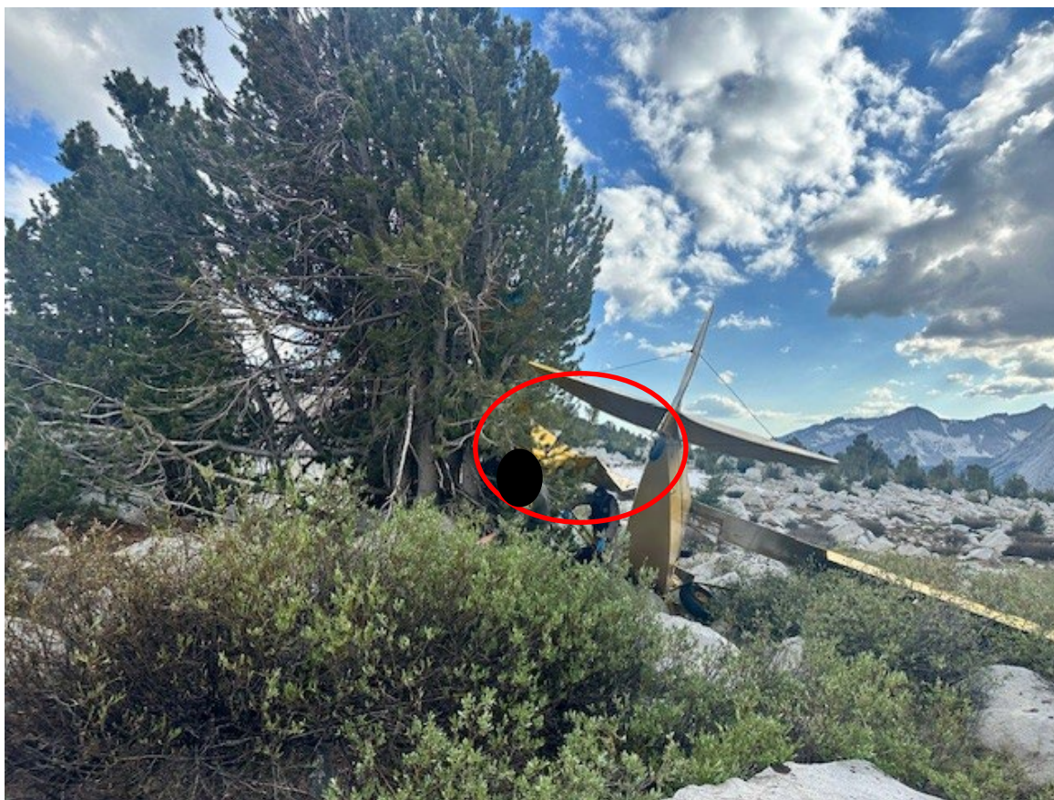
Photograph 2 - View of left wing damage (Courtesy of local law enforcement)
