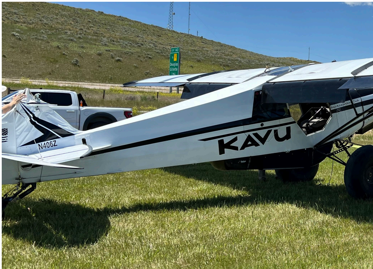
Photo 2 – Accident airplane after recovery; note damage to vertical stabilizer and rudder (courtesy of Federal Aviation Administration)
