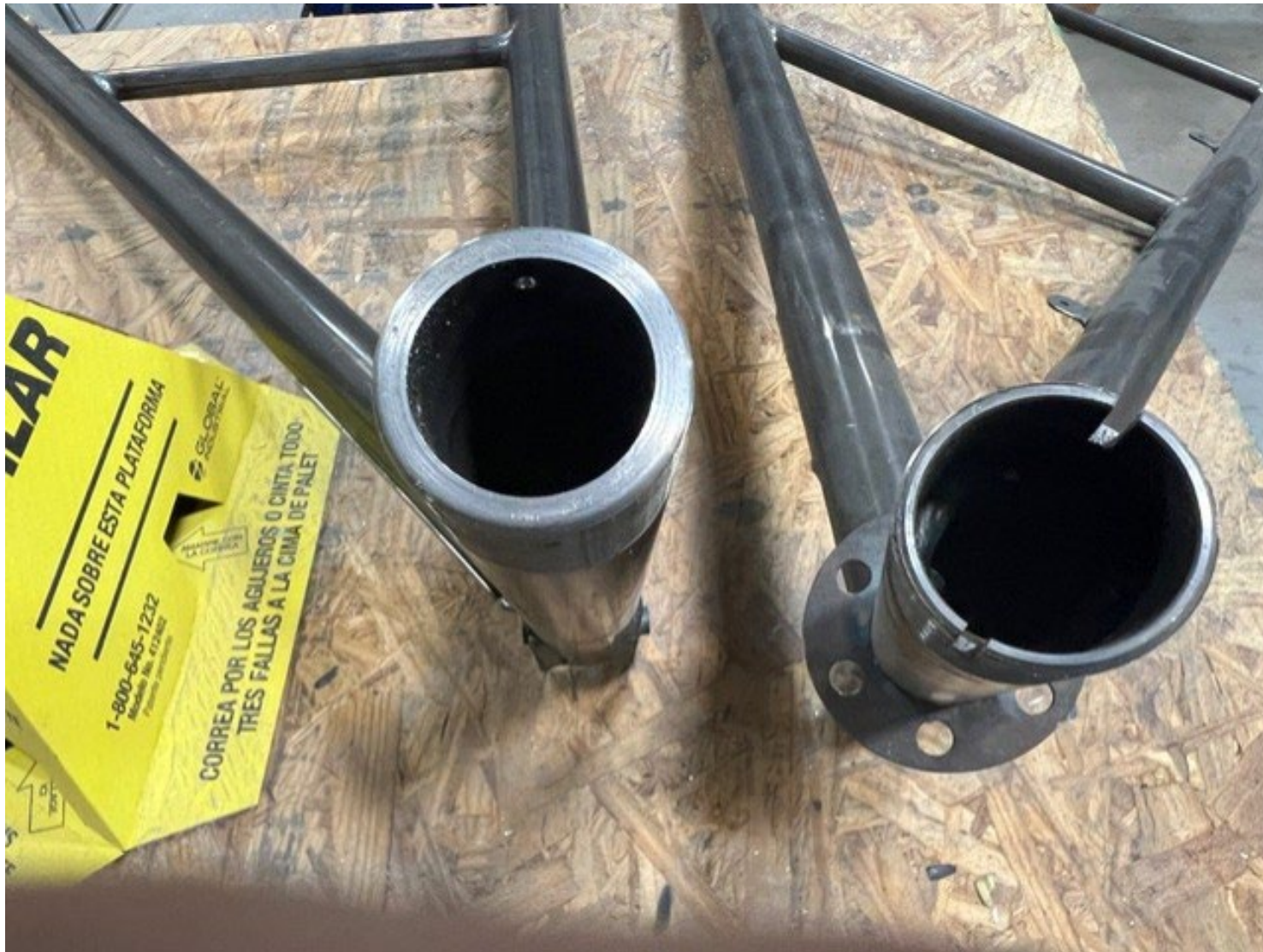
Photo 7 – Exemplar axles normally installed in Super Cubs (by Backcountry Super Cubs) (Courtesy of Backcountry Super Cubs)
