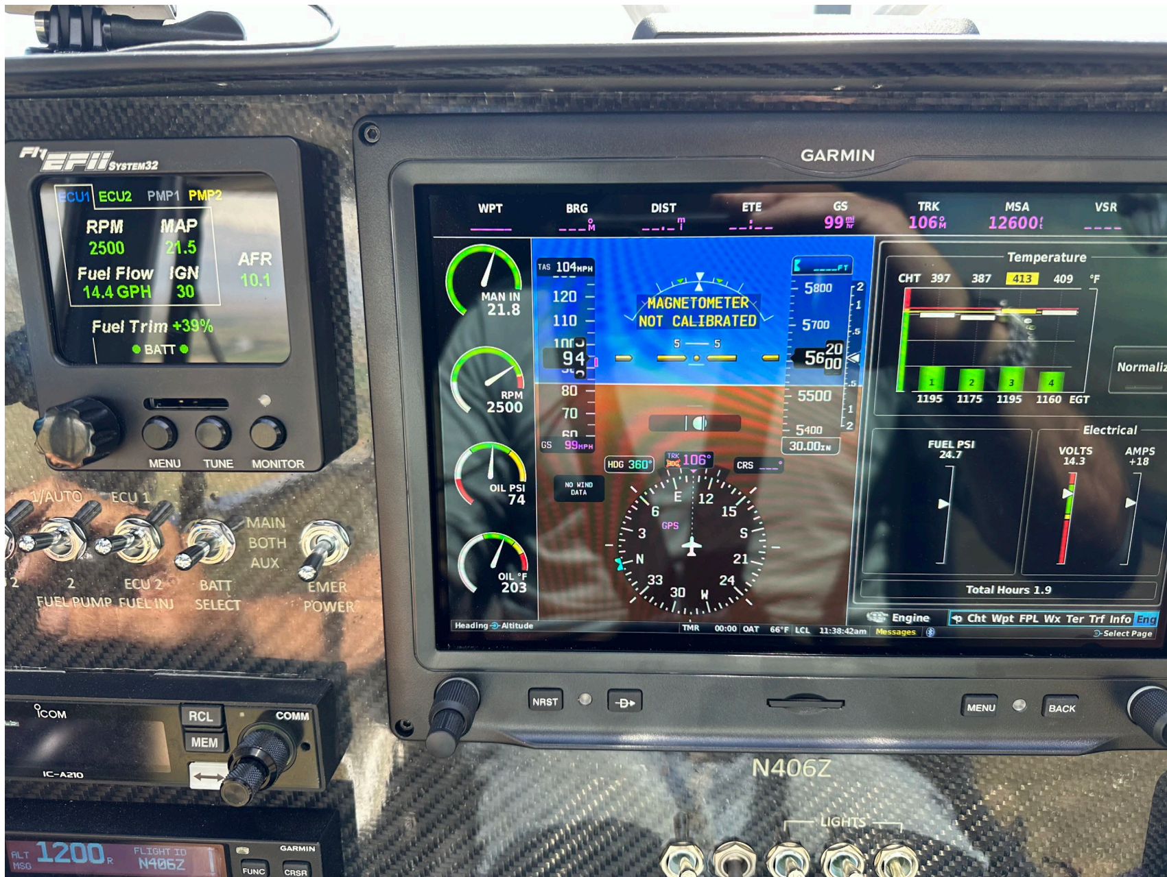
Photo 6 – EFII monitor and multi-function display during flight on June 21, 2024 (1138 lcl) (courtesy of accident pilot)
