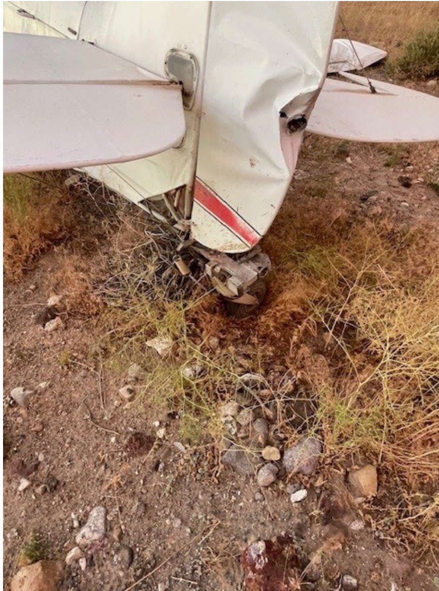
Photograph 2 - View of damage to rudder. (Courtesy of pilot)
