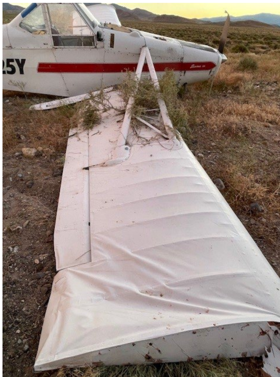
Photograph 1 - View of damage to right wing. (Courtesy of owner)
