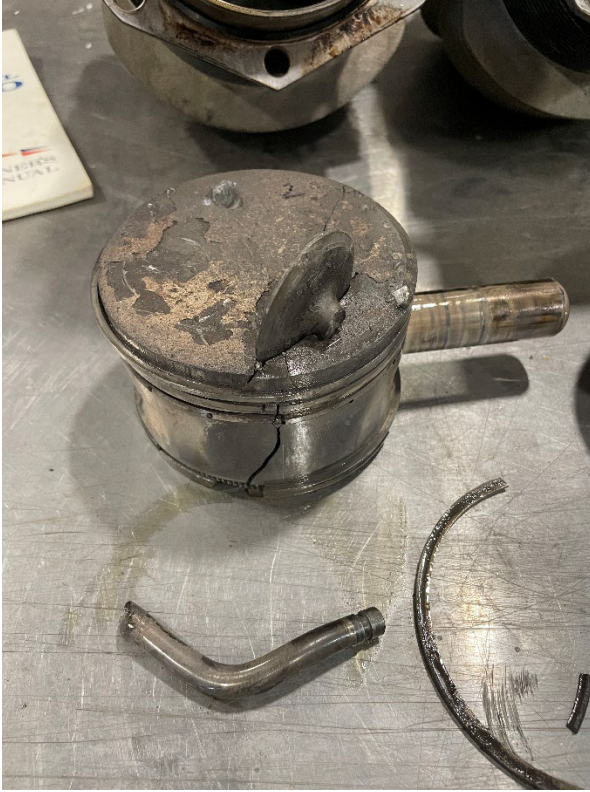
Figure 3- Intake valve head embedded in No. 2 piston head.
