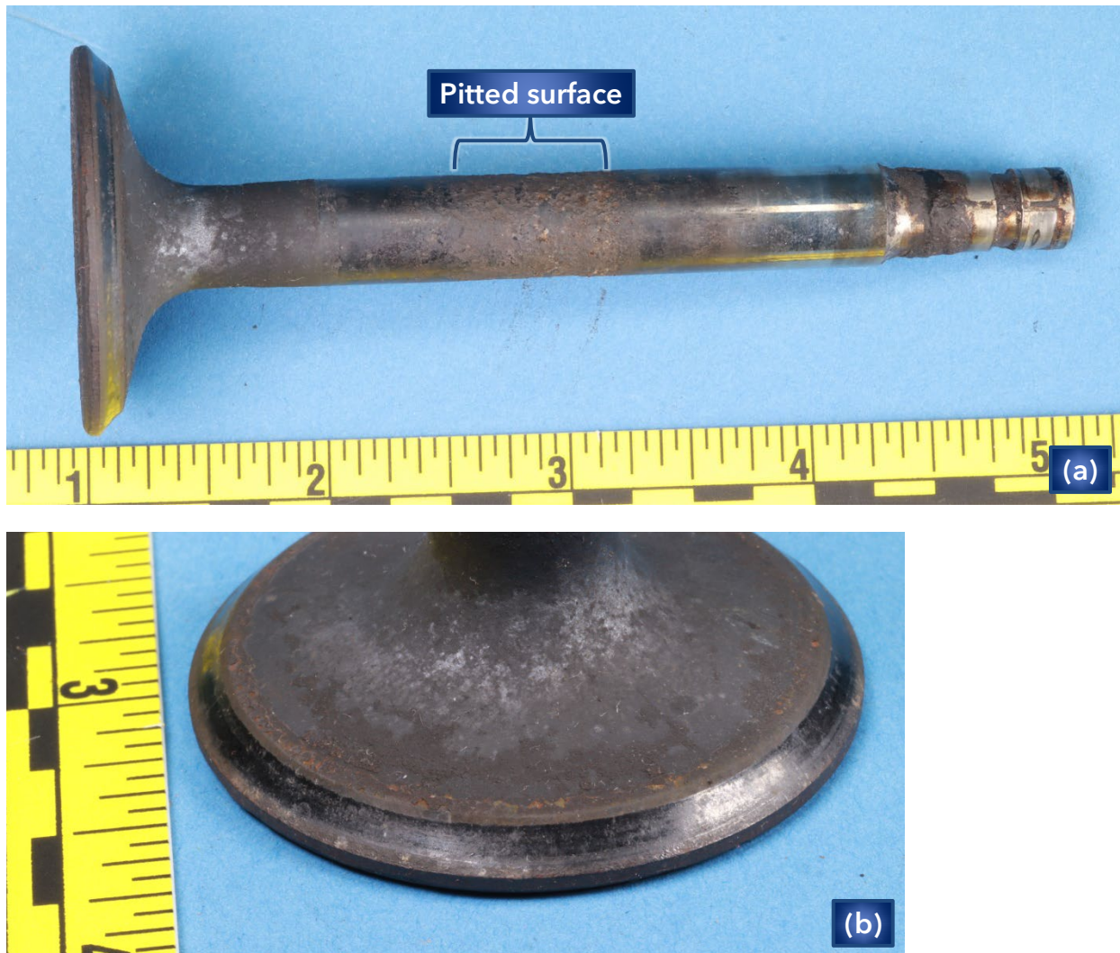
Figure 6. (a) Number 2 exhaust valve with (b) a close of the valve seat contact face.
