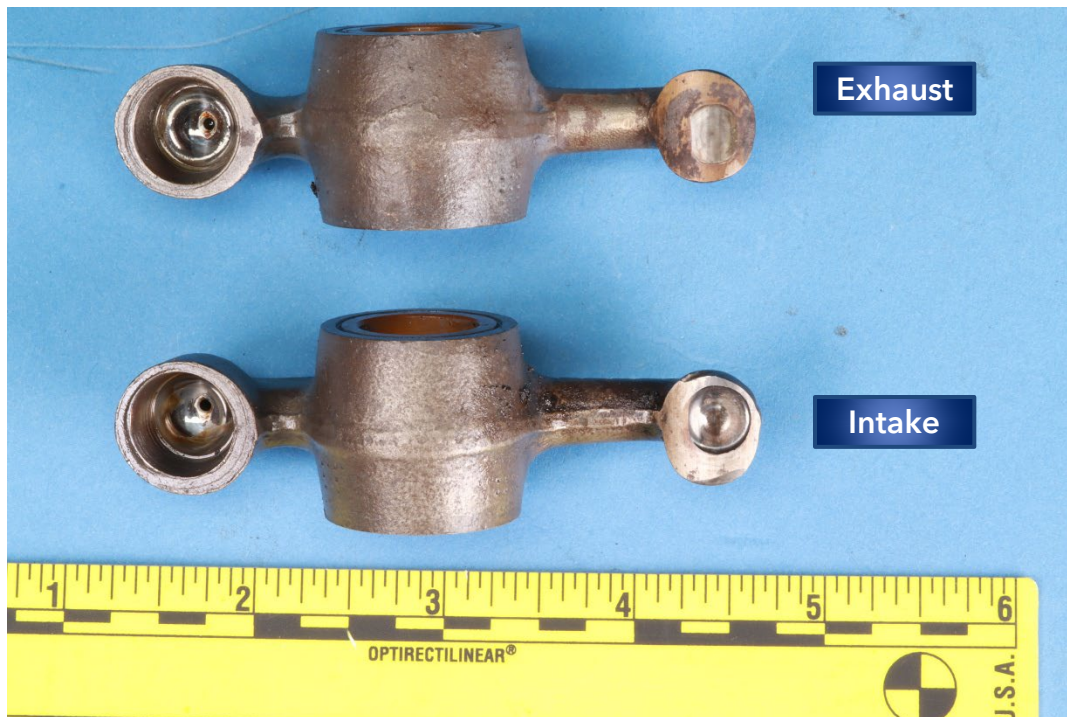
Figure 3. View of the rocker pads on the intake and exhaust rocker arms for the number 2 cylinder.
