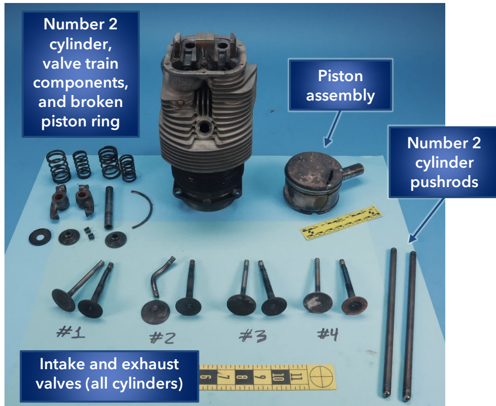
Figure 1. Overall view of the number 2 cylinder assembly including disassembled components from the valve train, number 2 piston assembly, and intake and exhaust valves for the remaining cylinders as received.
