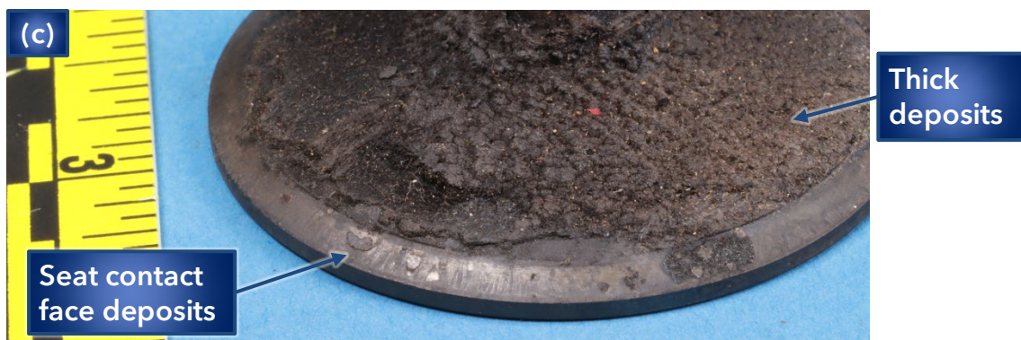
Figure 7. Number 4 intake valve (upper image) with closer views of a damaged area on the valve stem (middle image) and deposits on the stem side of the valve head including on the valve seat contact face (lower image).
