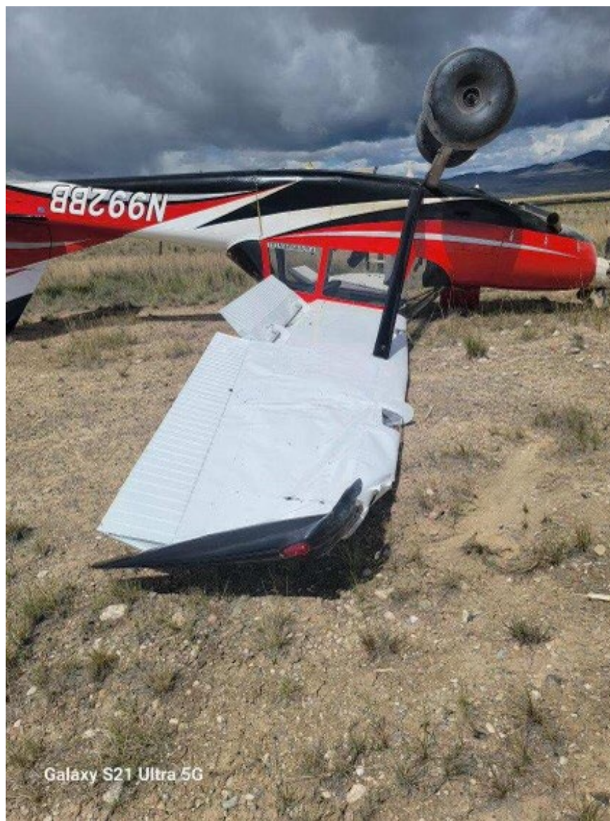
Photograph 1 - Aircraft inverted with left wing damage (Courtesy of the owner)
