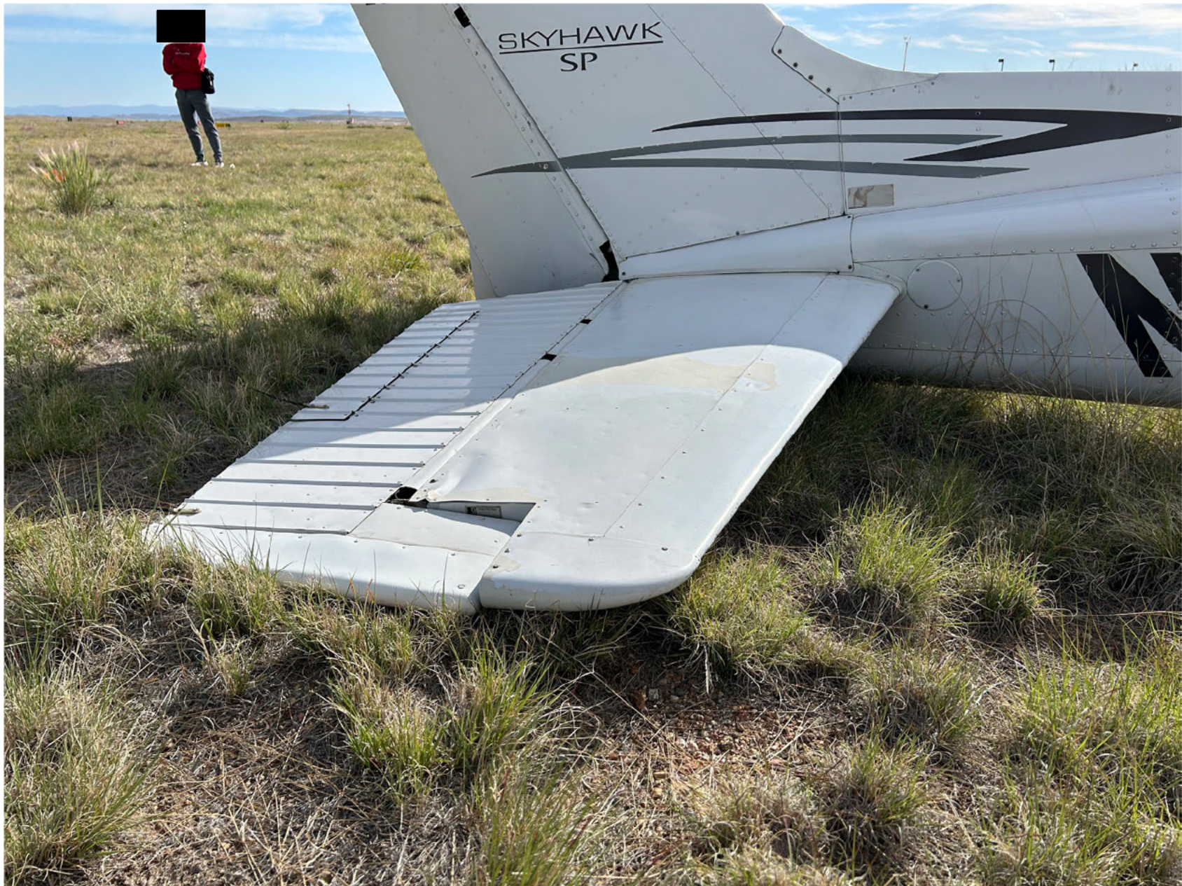
Photo 2 – Substantially damaged horizontal stabilizer. Photo courtesy of Airport Operations
