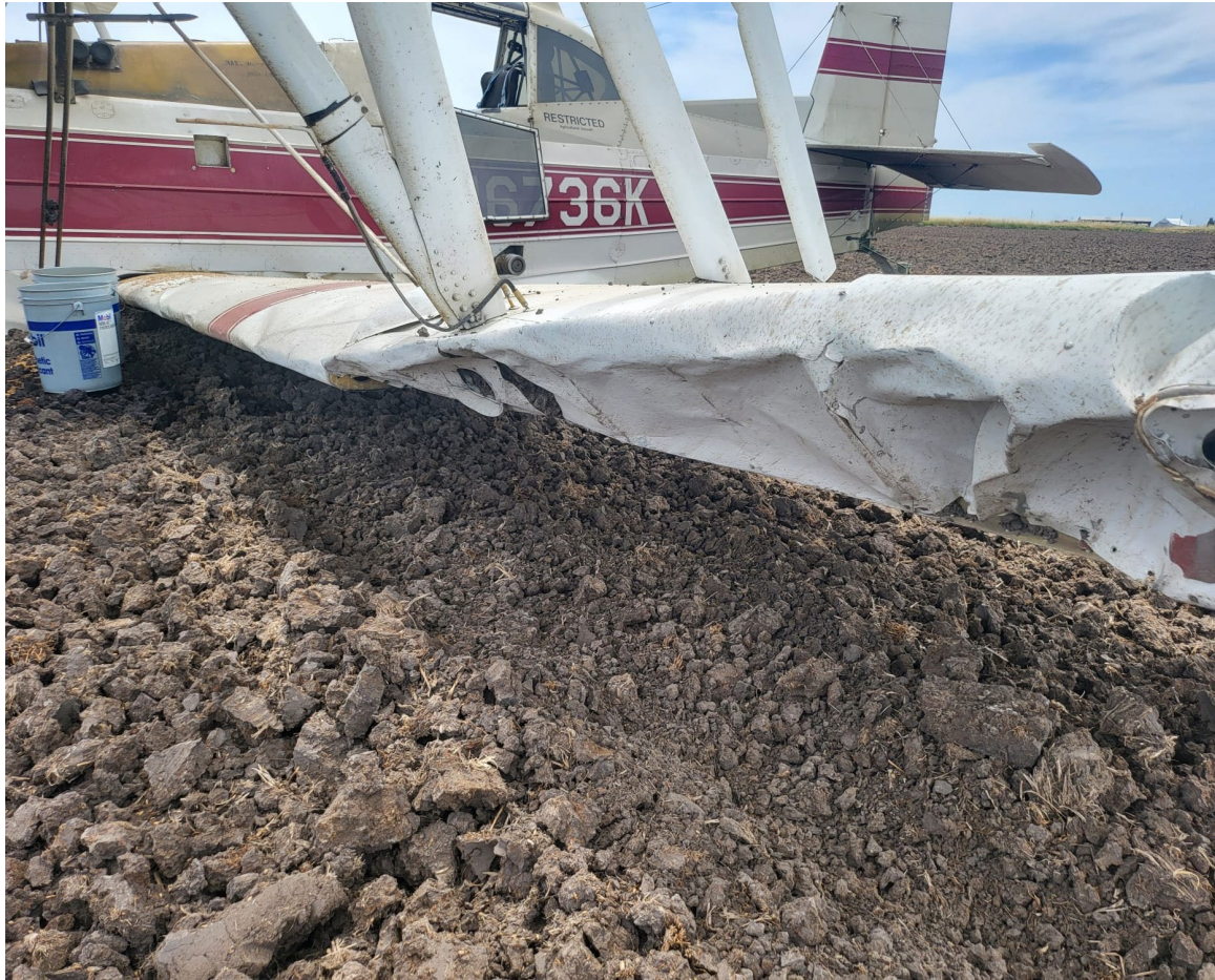
Photograph 3 - Left wing leading edge at accident site (Courtesy of the owner)
