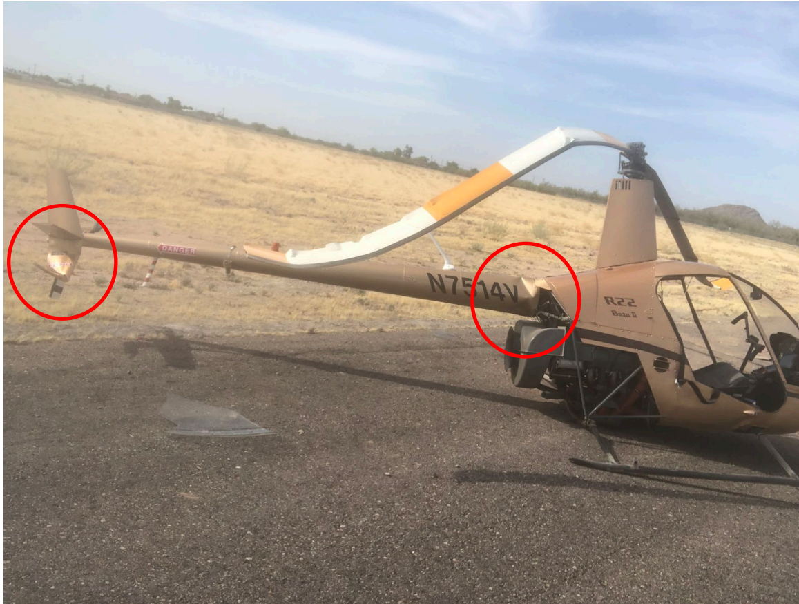
Photograph 2 - View of damage to tail boom and vertical stabilizer (Courtesy of Flight Instructor)
