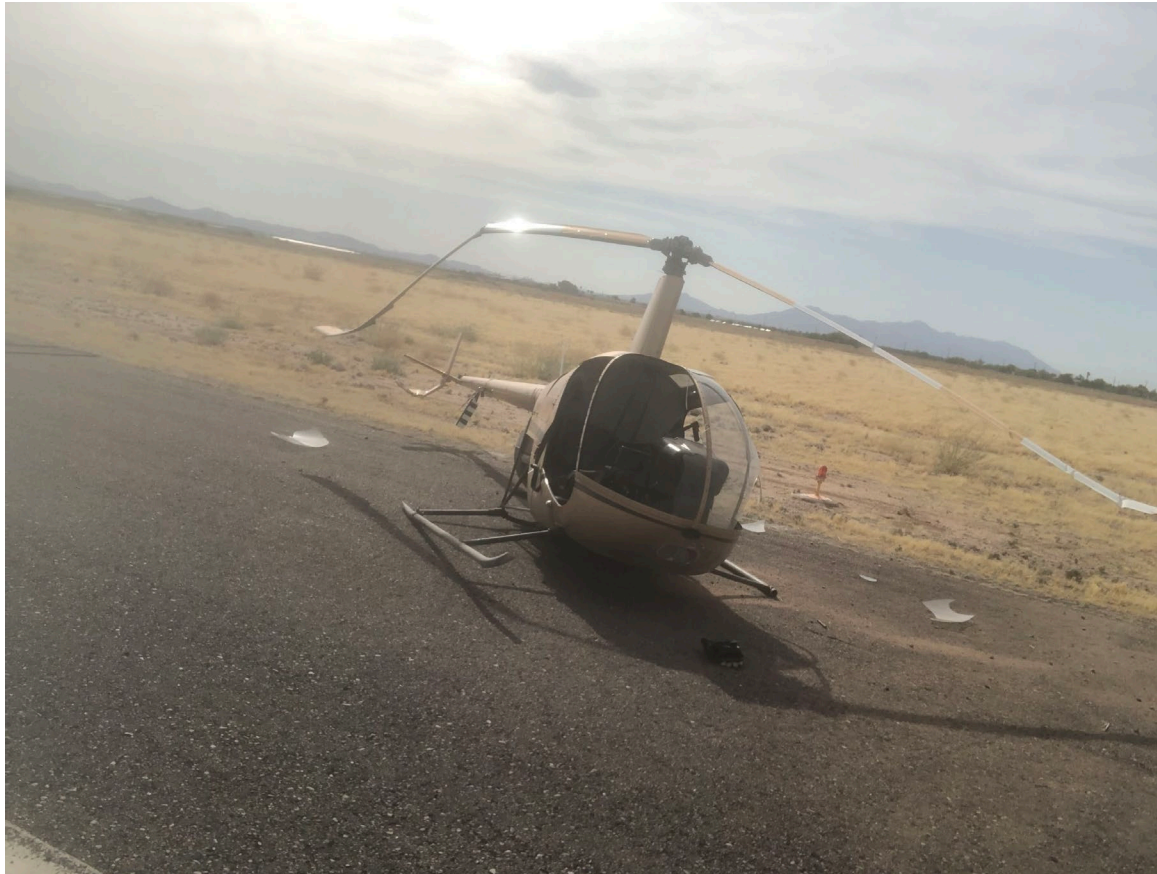
Photograph 1 - View of damage to main rotor blades (Courtesy of Flight Instructor)
