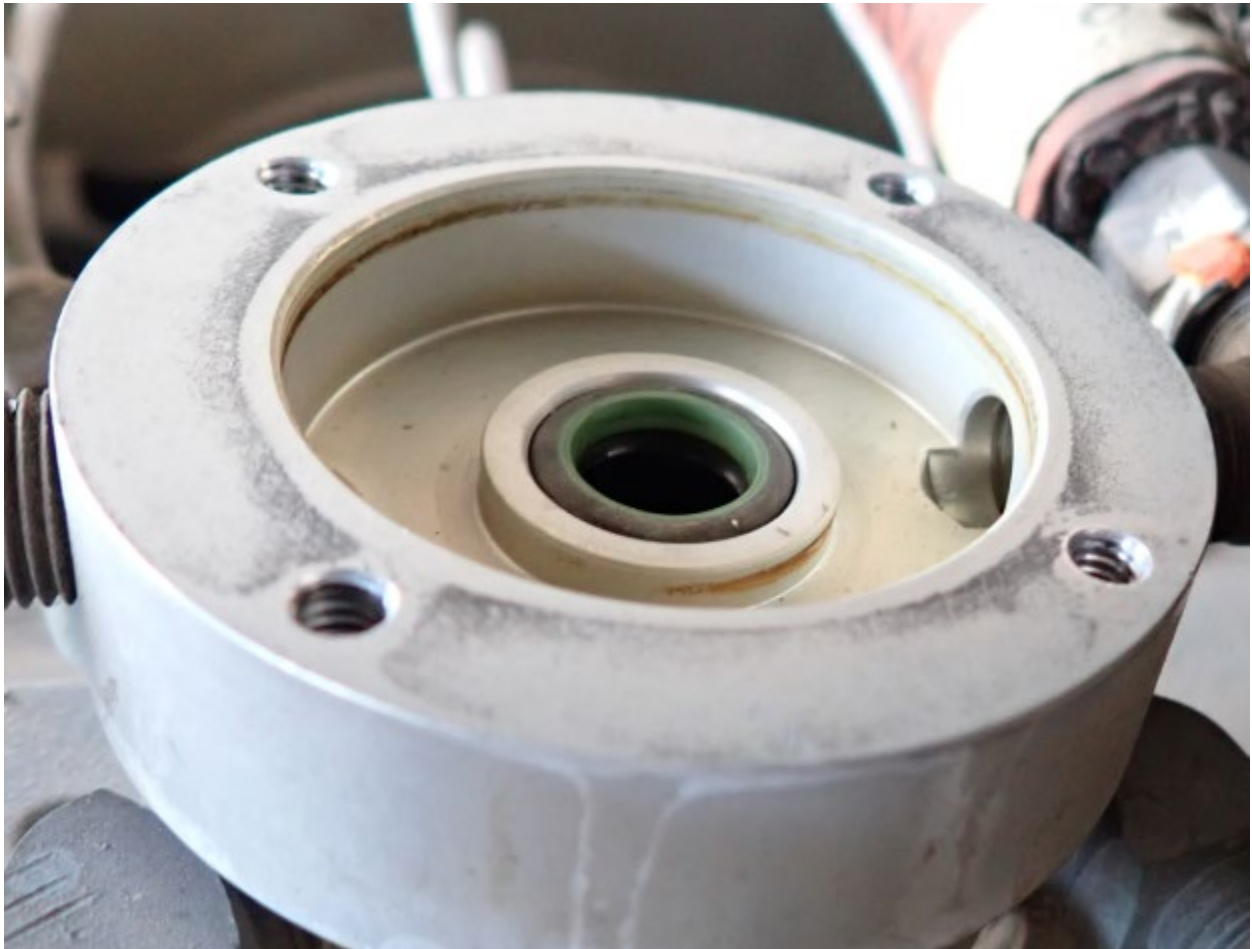
Figure 5: Manifold body (showing corrosion)
