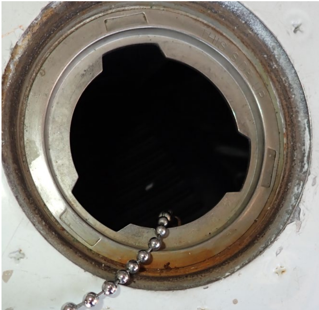
Figure 7: Fuel cap receptacle (showing corrosion)
