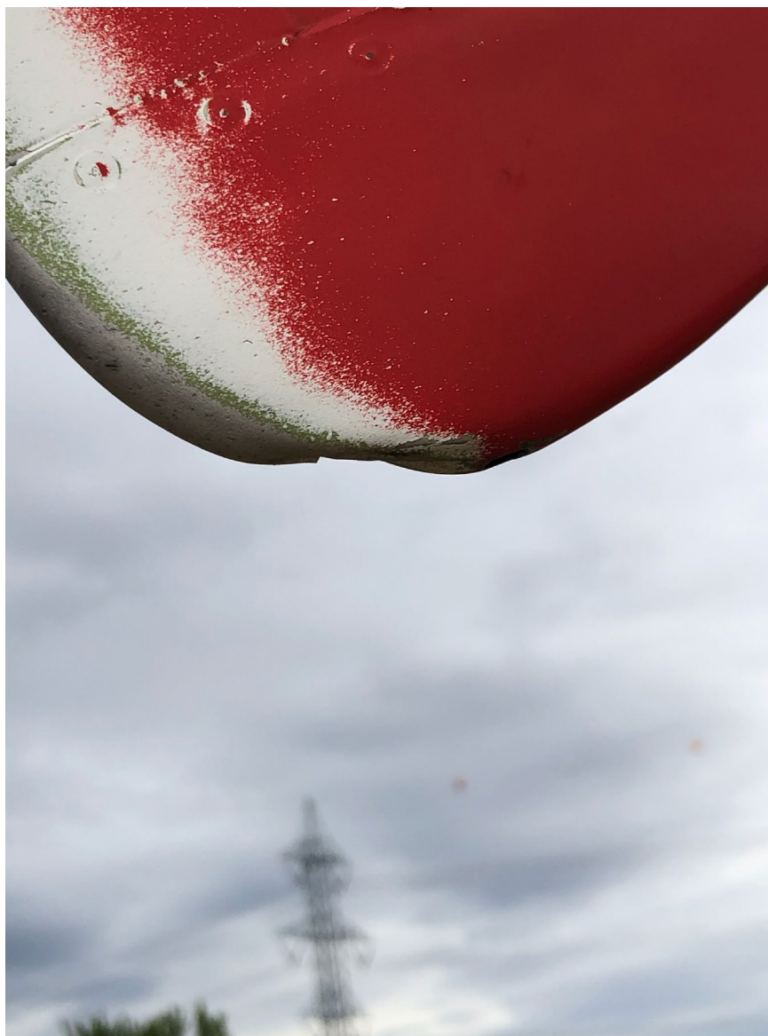
Photograph 2 - Close-up of tip damage (Courtesy of the operator)
