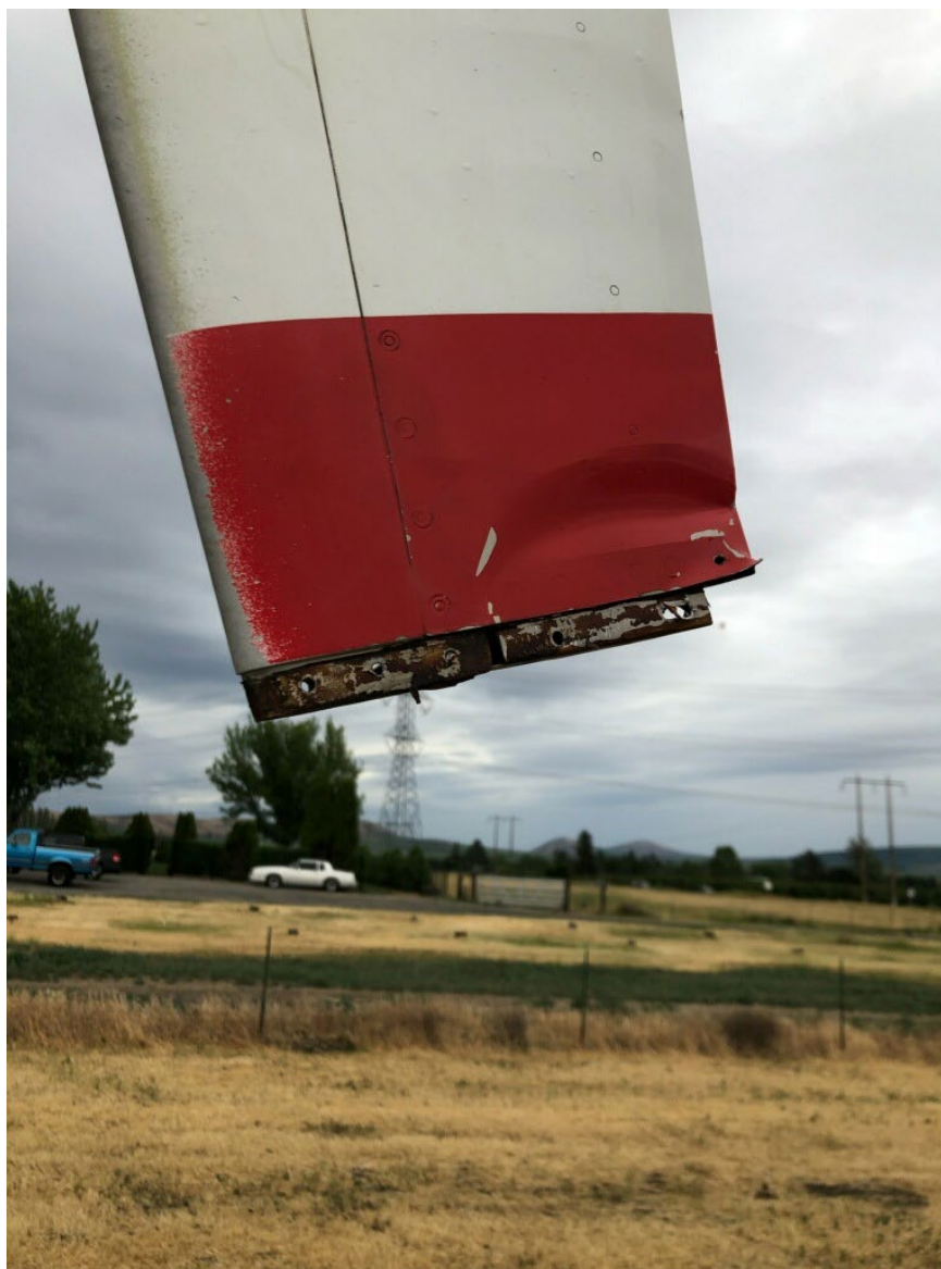
Photograph 3 - Close-up of tip and trailing edge damage (Courtesy of the operator)
