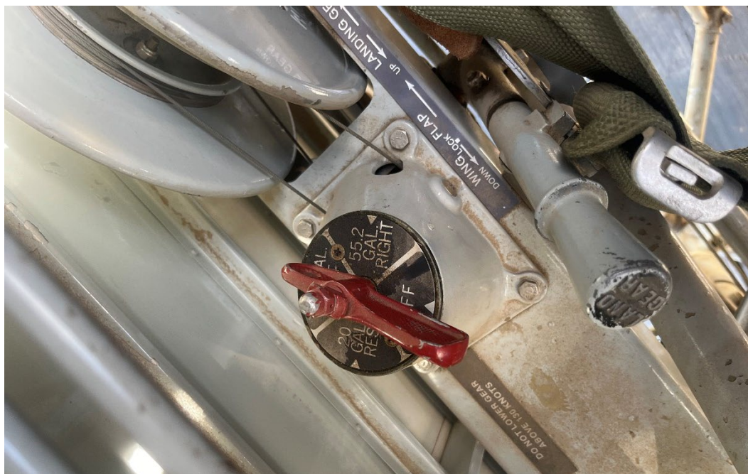
Figure 2: View of the fuel selector lever (Courtesy of recovery company)
