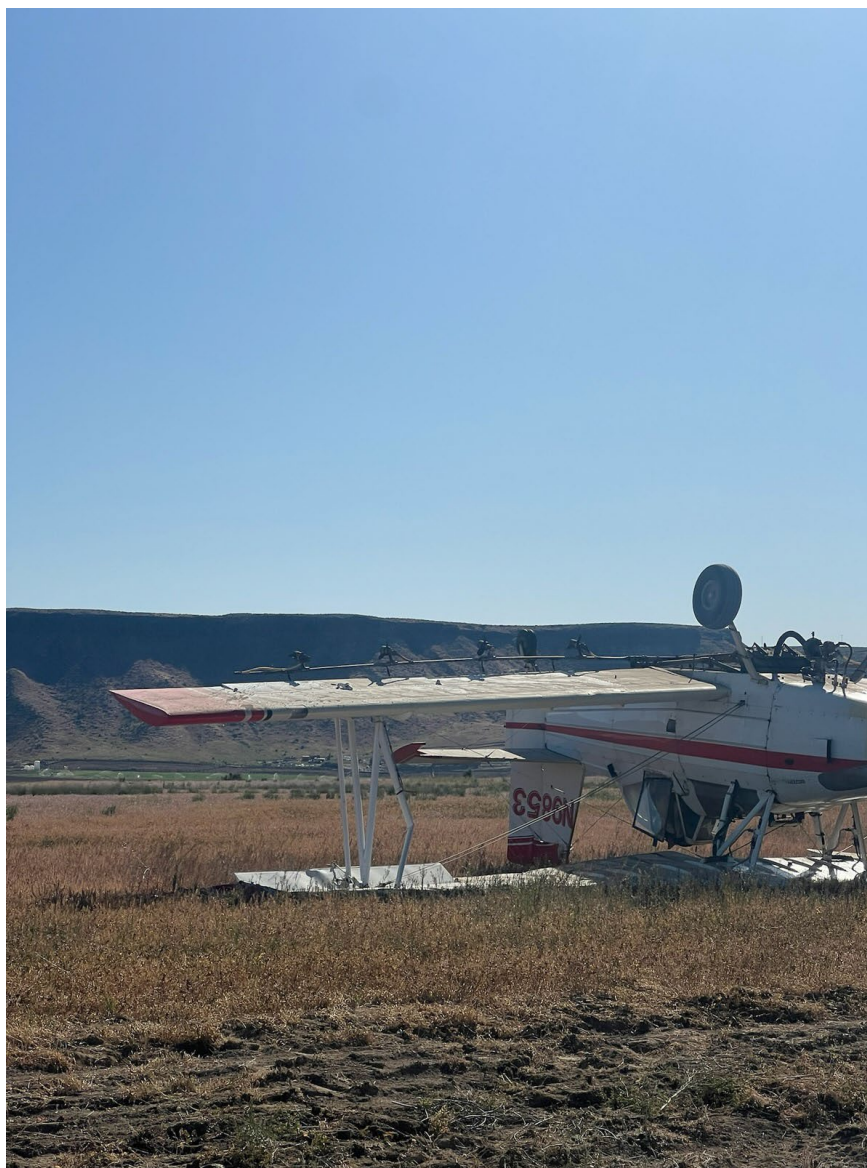
Photograph 3 - View of damage to upper wing. (Courtesy of pilot.)
