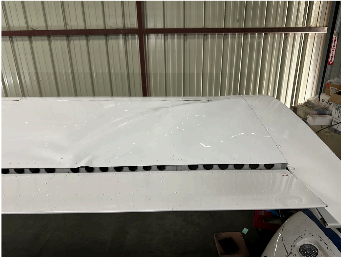
Photograph 1 - View of damage to right wing. (Courtesy of pilot)
