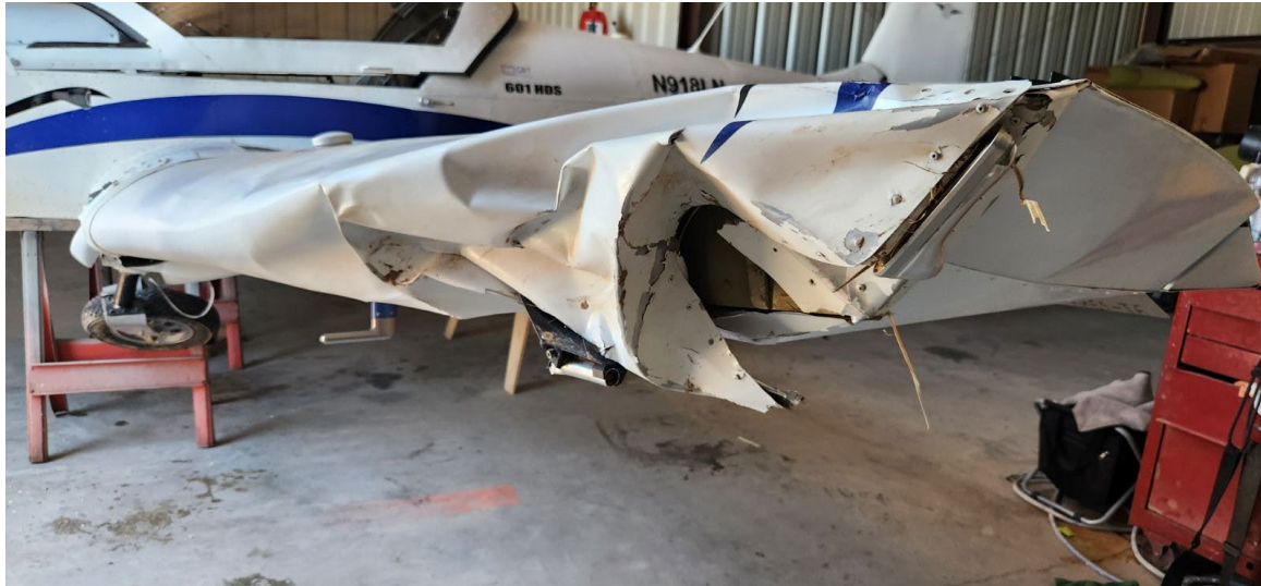
Photograph 2 - View of damage to left wing. (Courtesy of pilot)
