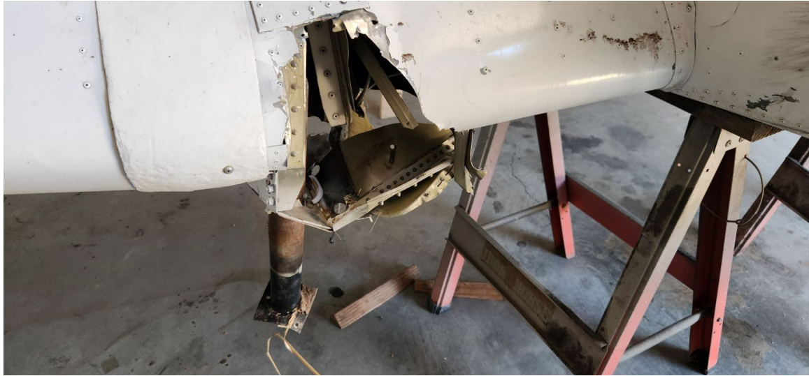
Photograph 3 - View of damage to right wing. (Courtesy of pilot.)
