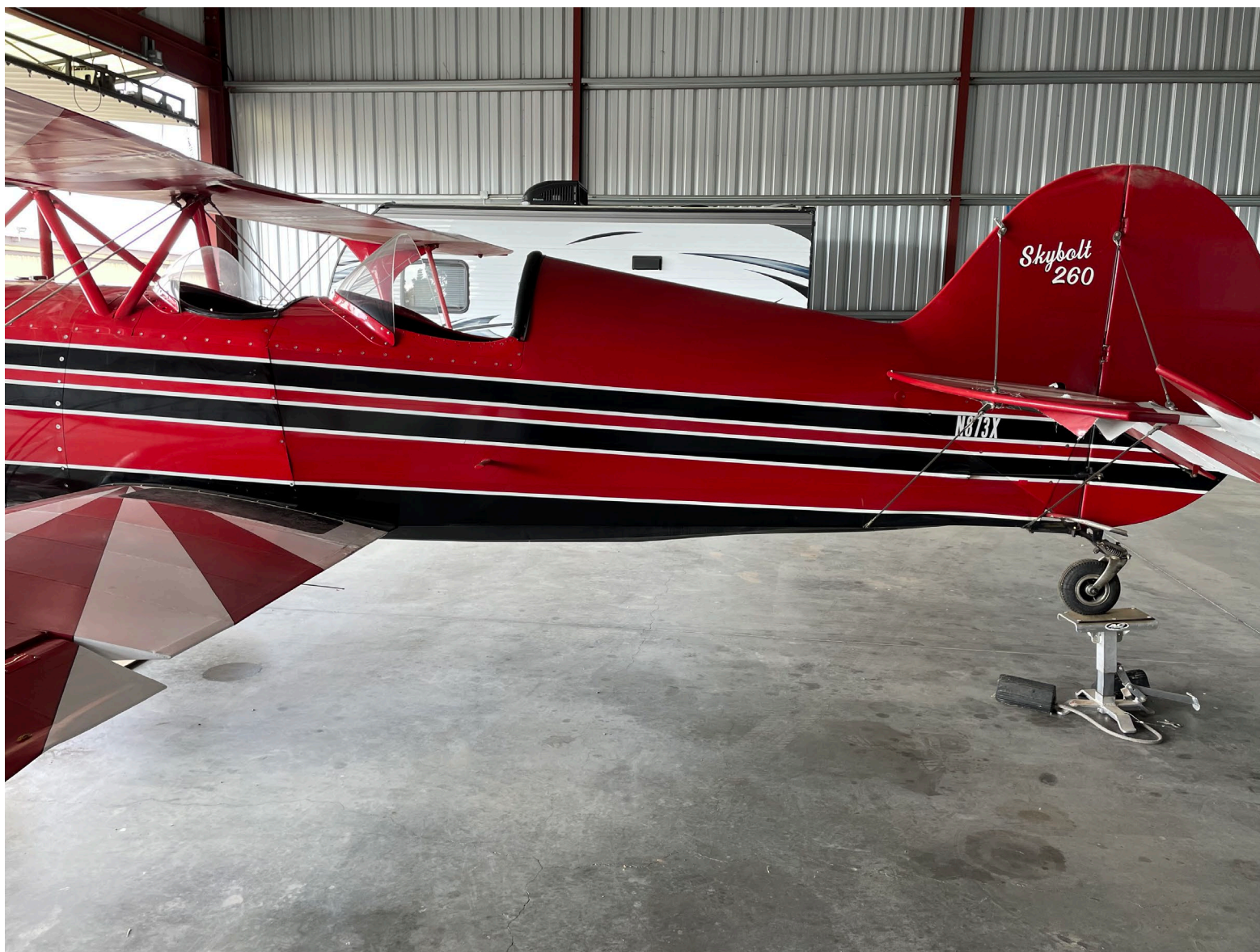
Photograph 2 - View of tail lifted for fuel test.
