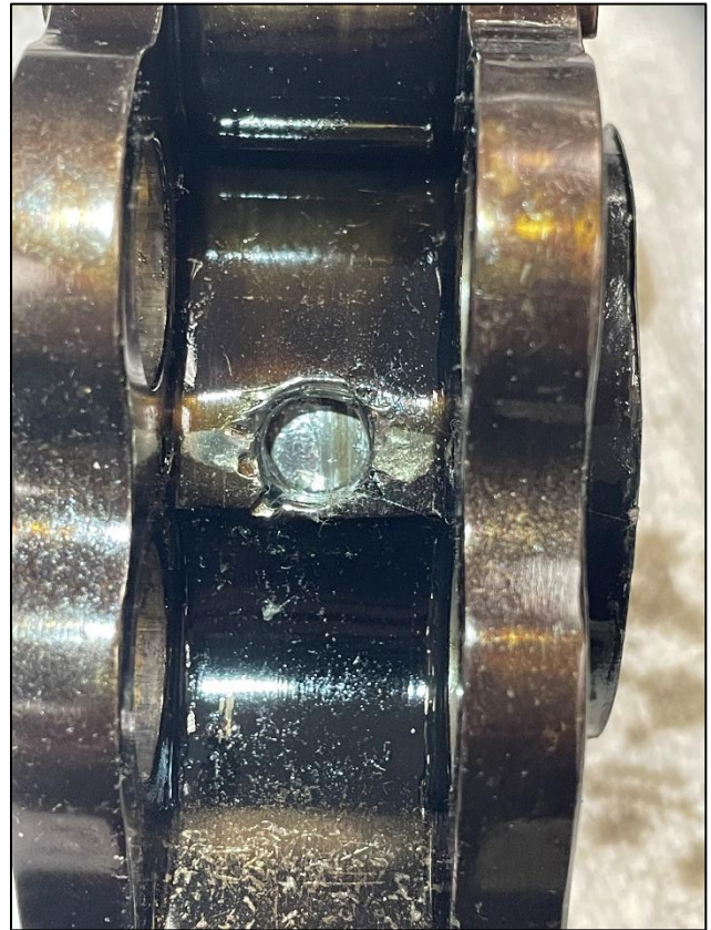
Figure 11-Master rod main bearing set screw hole and installation strike marks.
