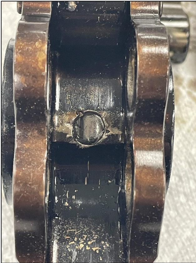
Figure 10-Master rod main bearing set screw hole and installation strike marks.
