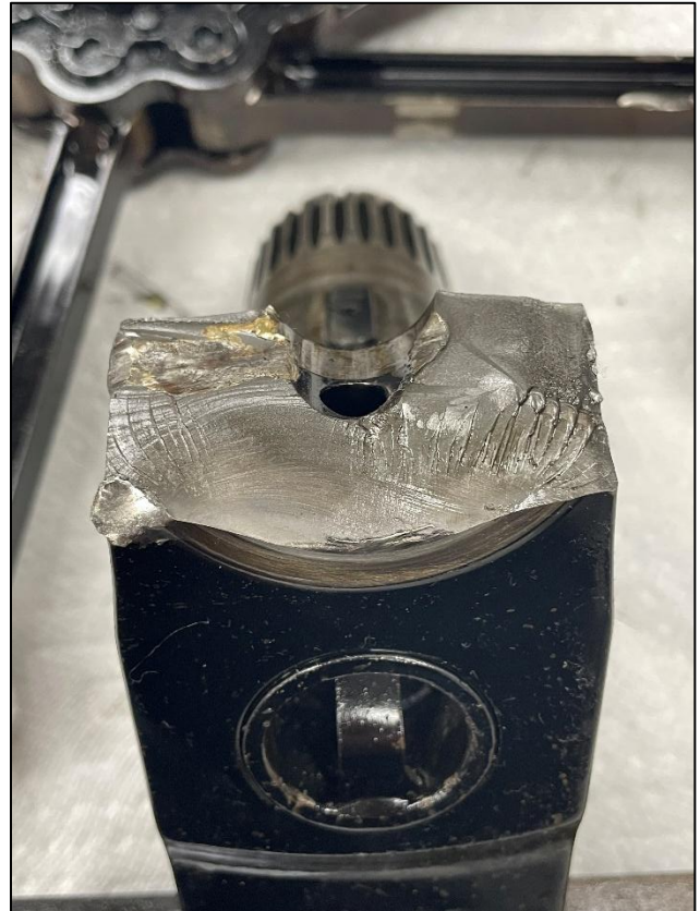
Figure 14-Crankshaft forward section separation surface.
