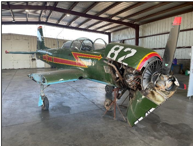
Figure 1-Main wreckage and engine.
