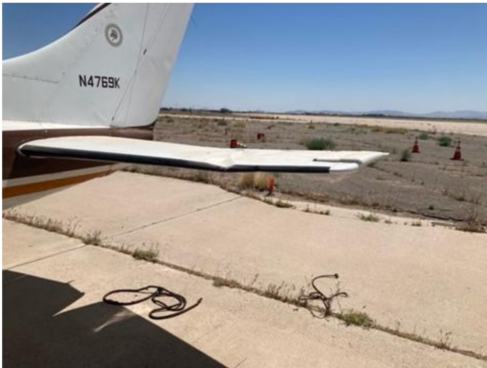
Photograph 4 - Left horizontal stabilizer and elevator damage. (Courtesy of the Mechanic)
