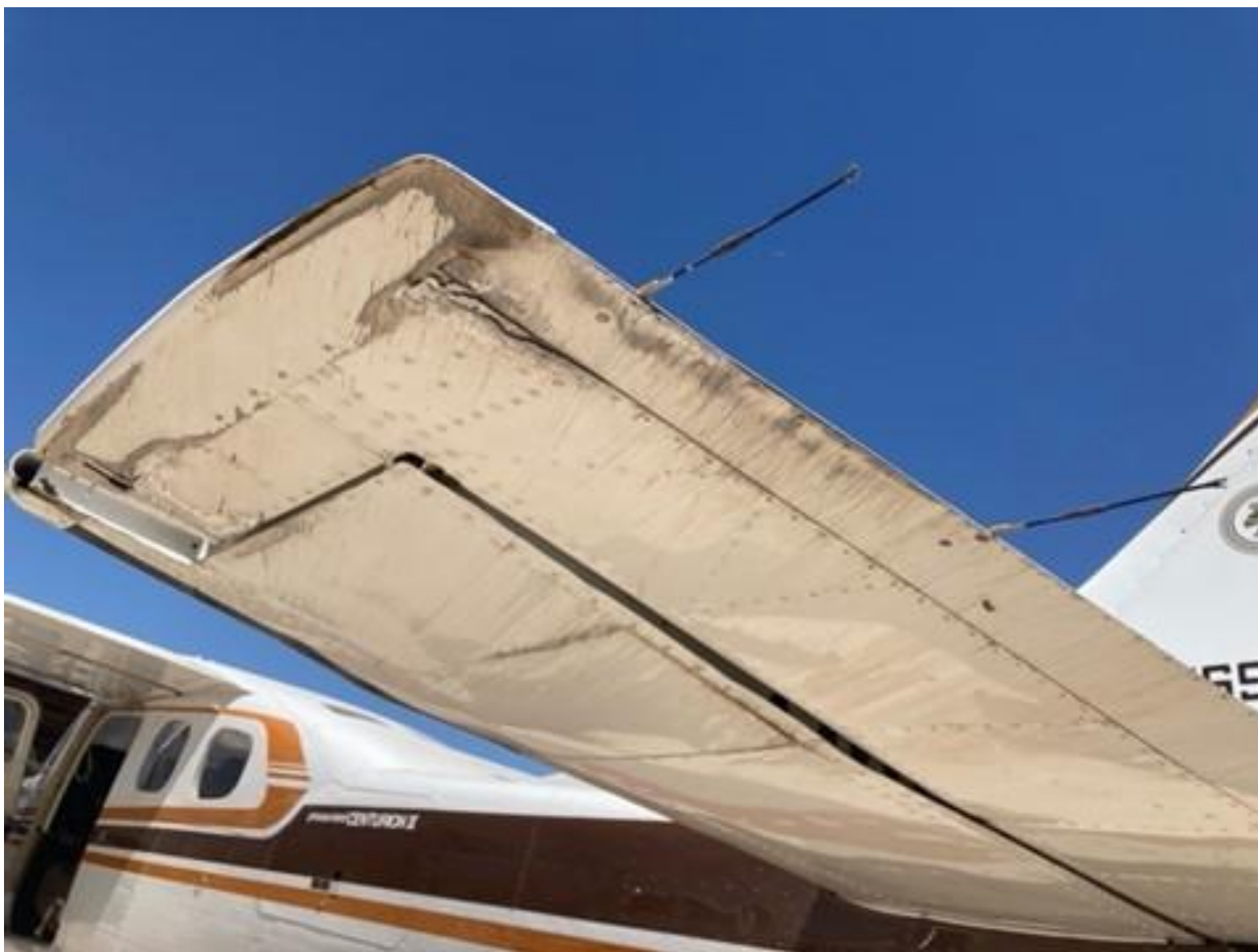
Photograph 5 - Left horizontal stabilizer and elevator damage. (Courtesy of the Mechanic)
