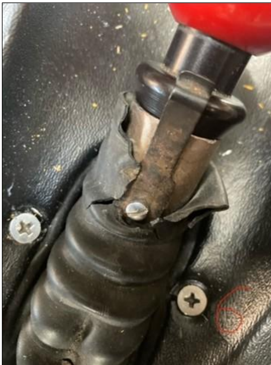
Photograph 3 - Landing gear emergency extension handle. (Courtesy of the Mechanic)
