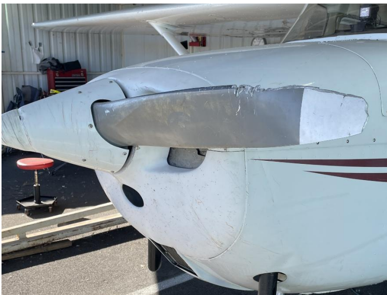
Figure 6: View of Propeller Blade Note Damage
