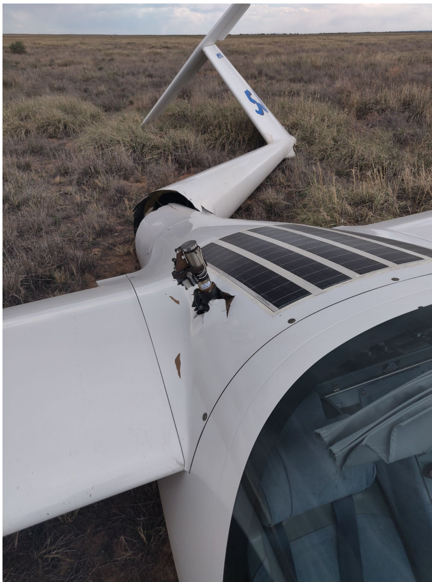
Photograph 2 - View of aft fuselage damage. (Courtesy of airport manager.)
