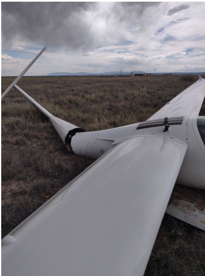
Photograph 3 - View of empennage damage. (Courtesy of airport manager)
