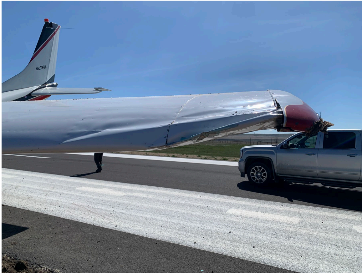
Photograph 3 - View of damage to the left wing. (Courtesy of pilot)
