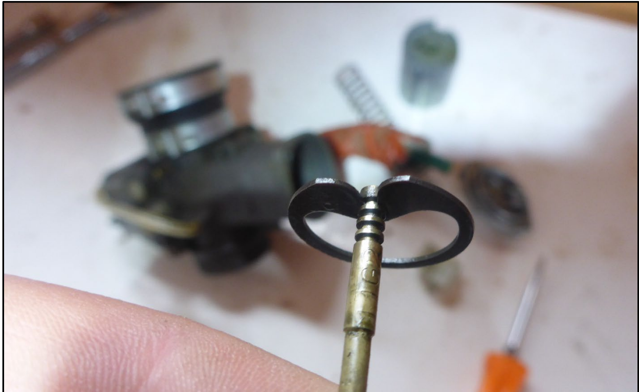
Photograph 2: The MAG carburetor needle clip in the number 1 (most lean position).
