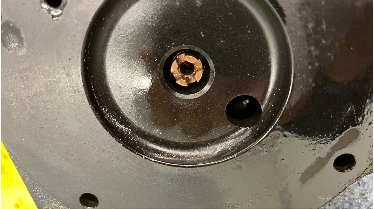
Figure 4 - Non-ferrous particles on the fuel-side plate
