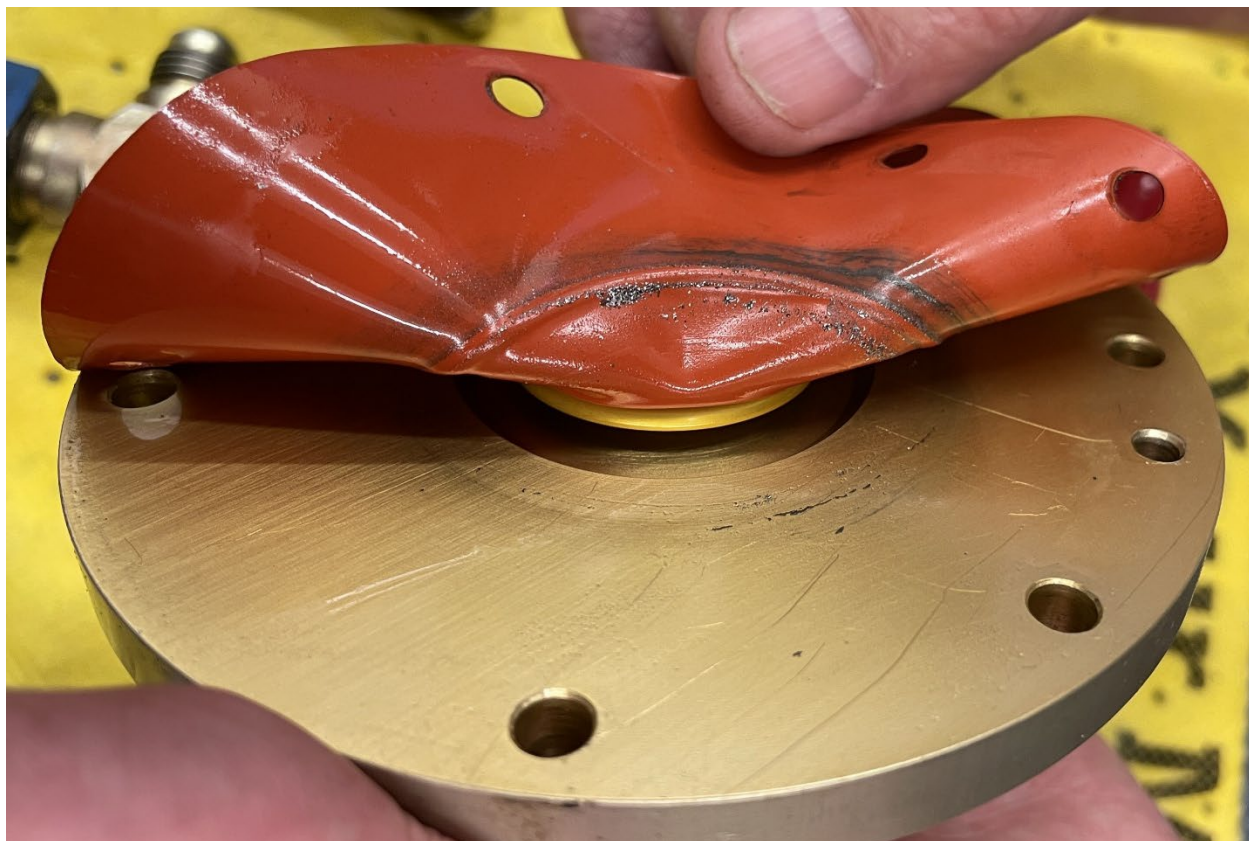
Figure 3 - Non-ferrous particles on the fuel-side diaphragm surface
