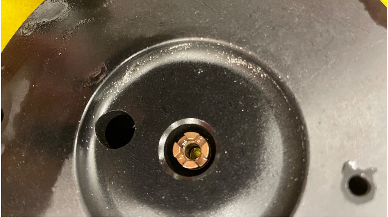
Figure 6 - Non-ferrous particles on the body inner surface
