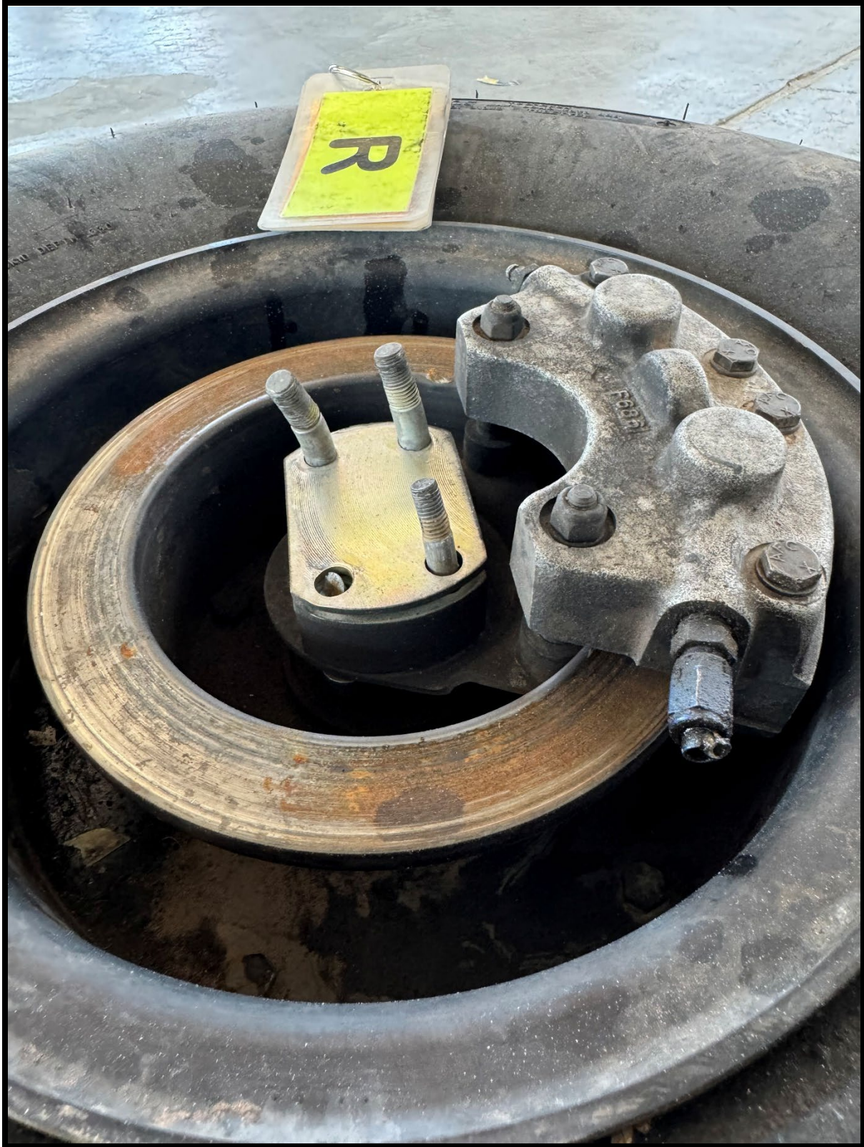
Figure 2: Close up view of the separated right main landing gear wheel and caliper with impact damage to hydraulic line AN fitting, and deformation to axle attachment bolts.
