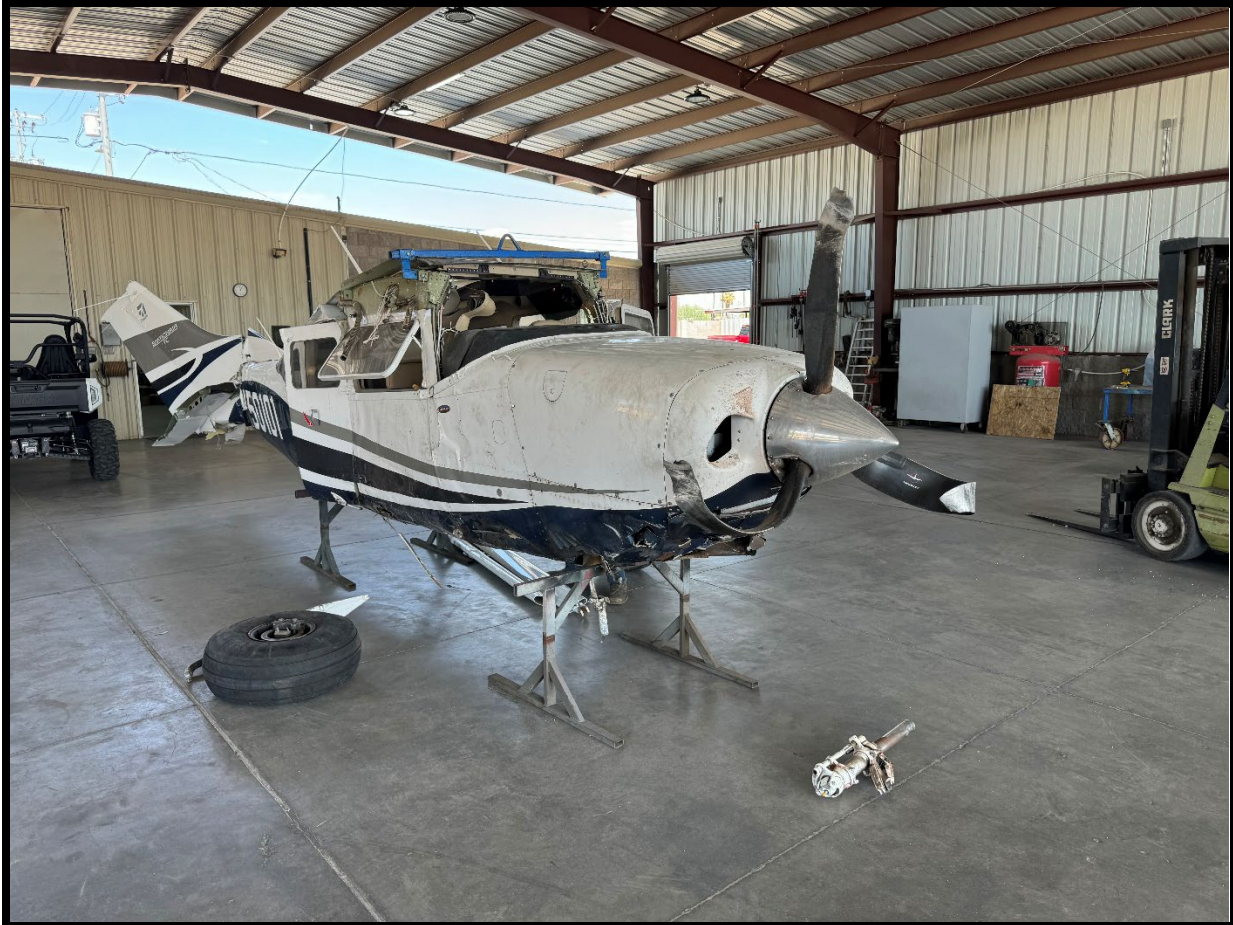
Figure 1: Forward right side view of the airplane with impact separated nose landing gear and right main landing gear.
