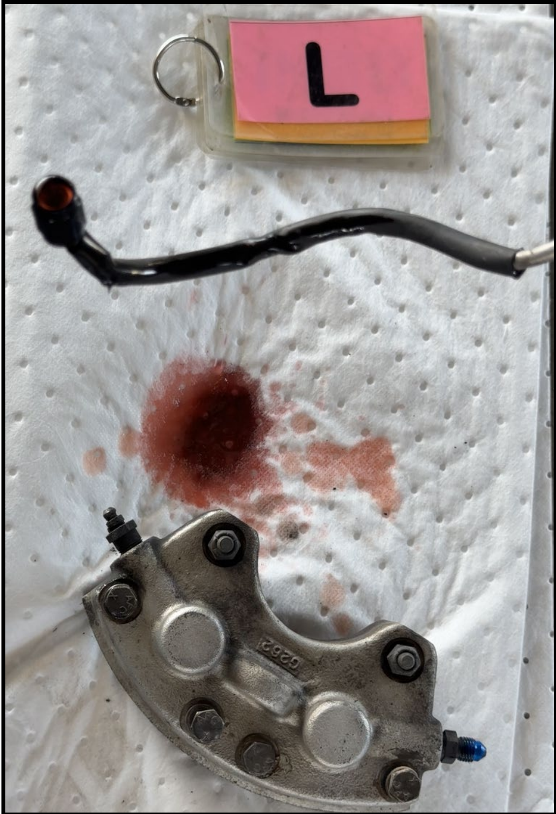
Figure 10: Left main gear hydraulic brake line function test showing fluid pressure at AN fitting body.
