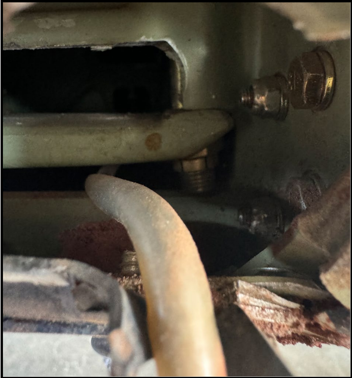
Figure 7: Close up view of left main landing gear spring forward channel separation.
