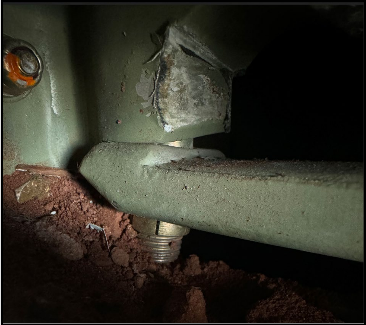
Figure 6: Close up view of left main landing gear spring aft channel separation.
