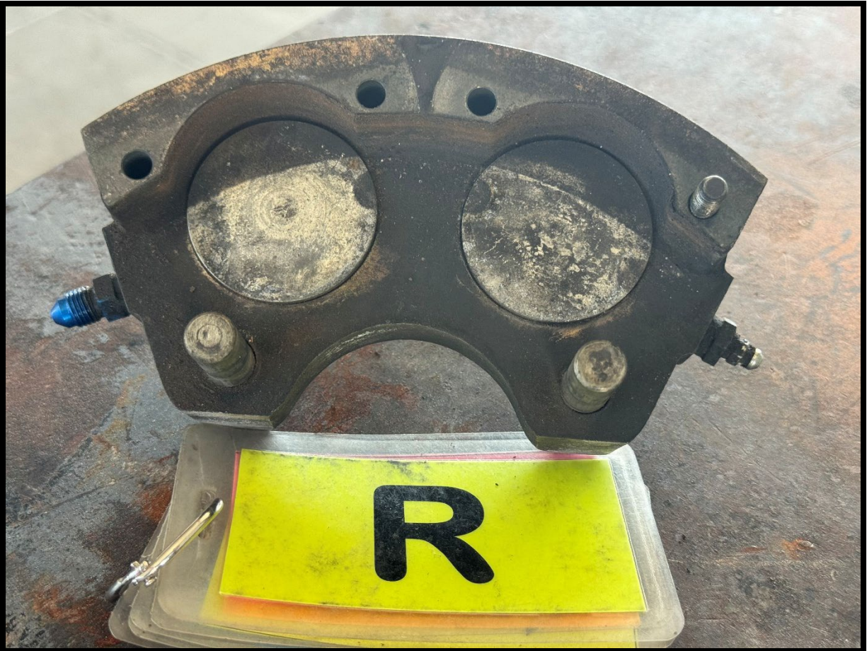
Figure 15: Close up view of right main landing gear brake caliper pistons with pressure plate removed.
