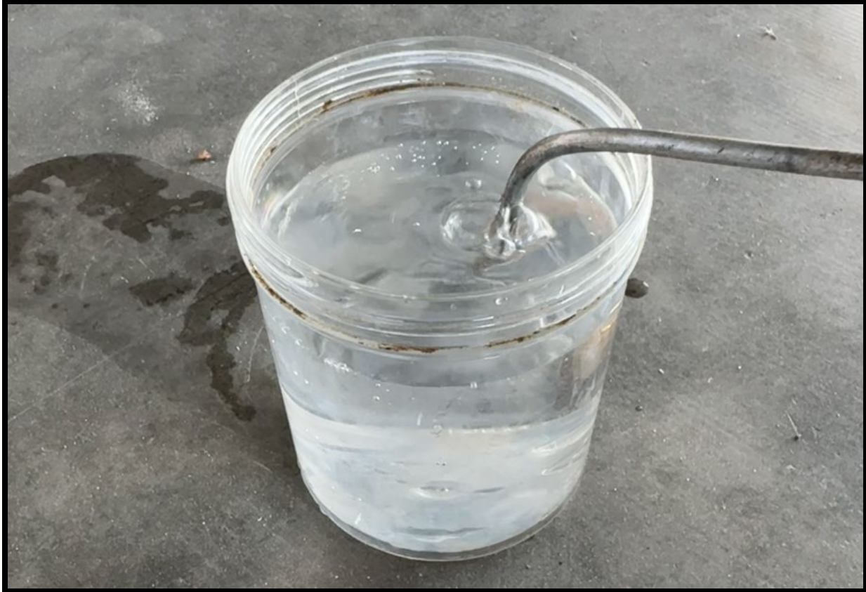
Figure 9: Right hydraulic brake line function test showing mason jar and bubble production, pressure indication.
