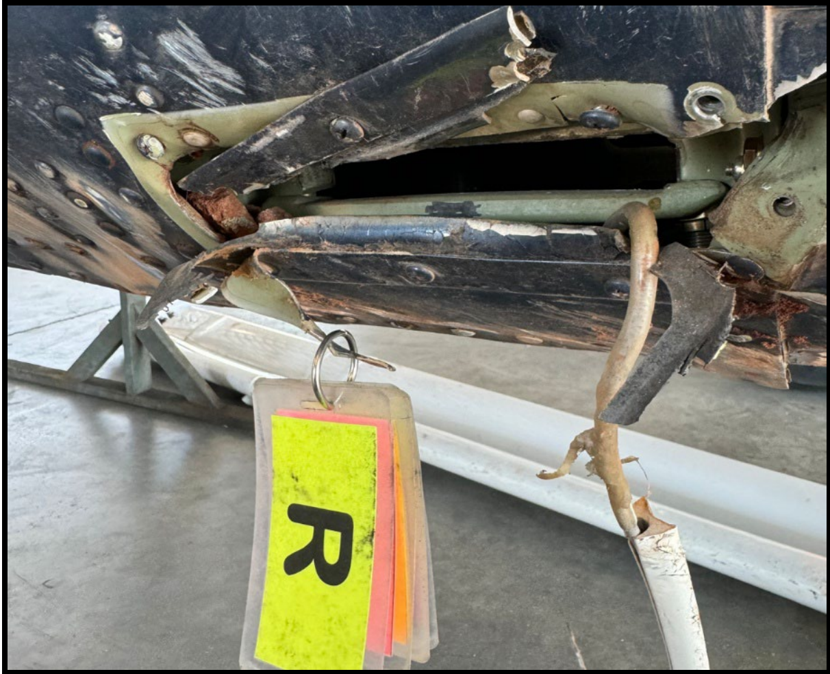
Figure 5: Initial view of right main landing gear spring lower fuselage separation.
