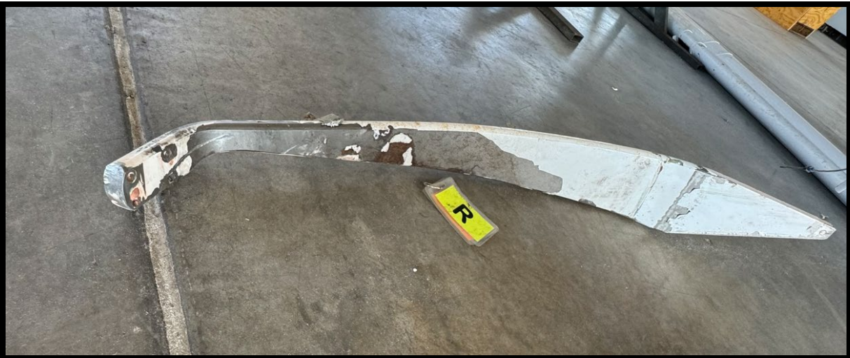
Figure 4: Bottom to top view of impact separated right main landing gear spring
