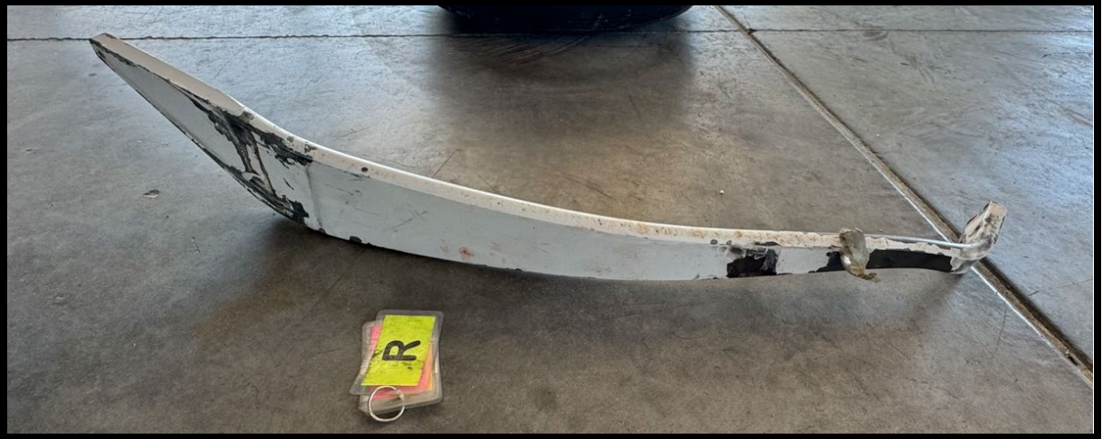
Figure 3: Top to bottom view of impact separated right main landing gear spring
