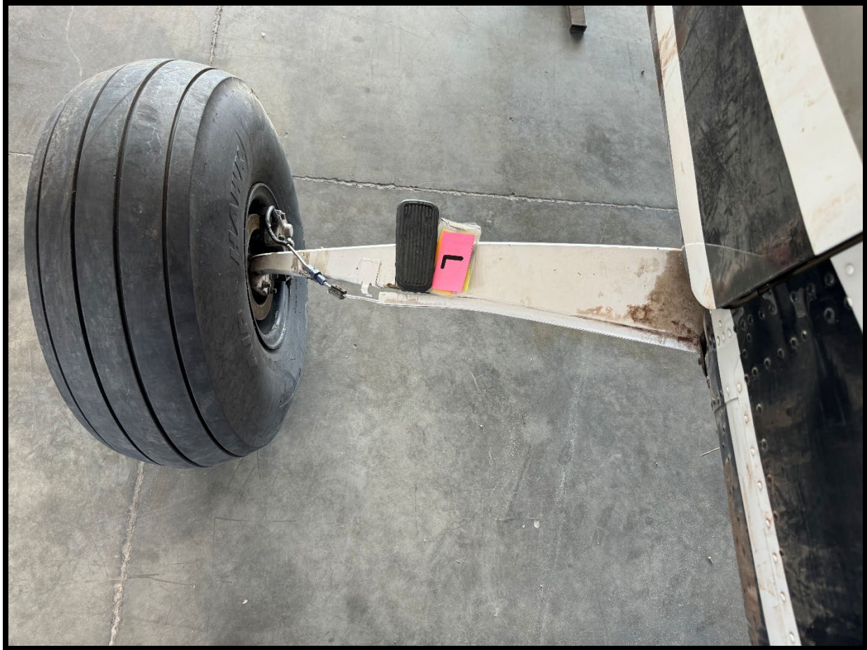
Figure 8: Initial view of the left main landing gear, connected hydraulic fluid line and caliper.
