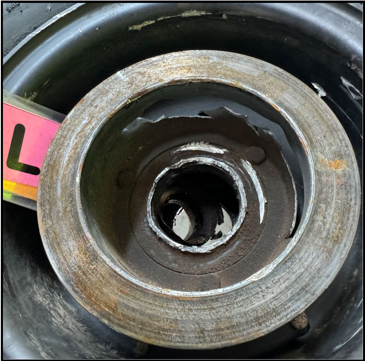
Figure 12: View damage to the left wheel inner half and bearing assembly.
