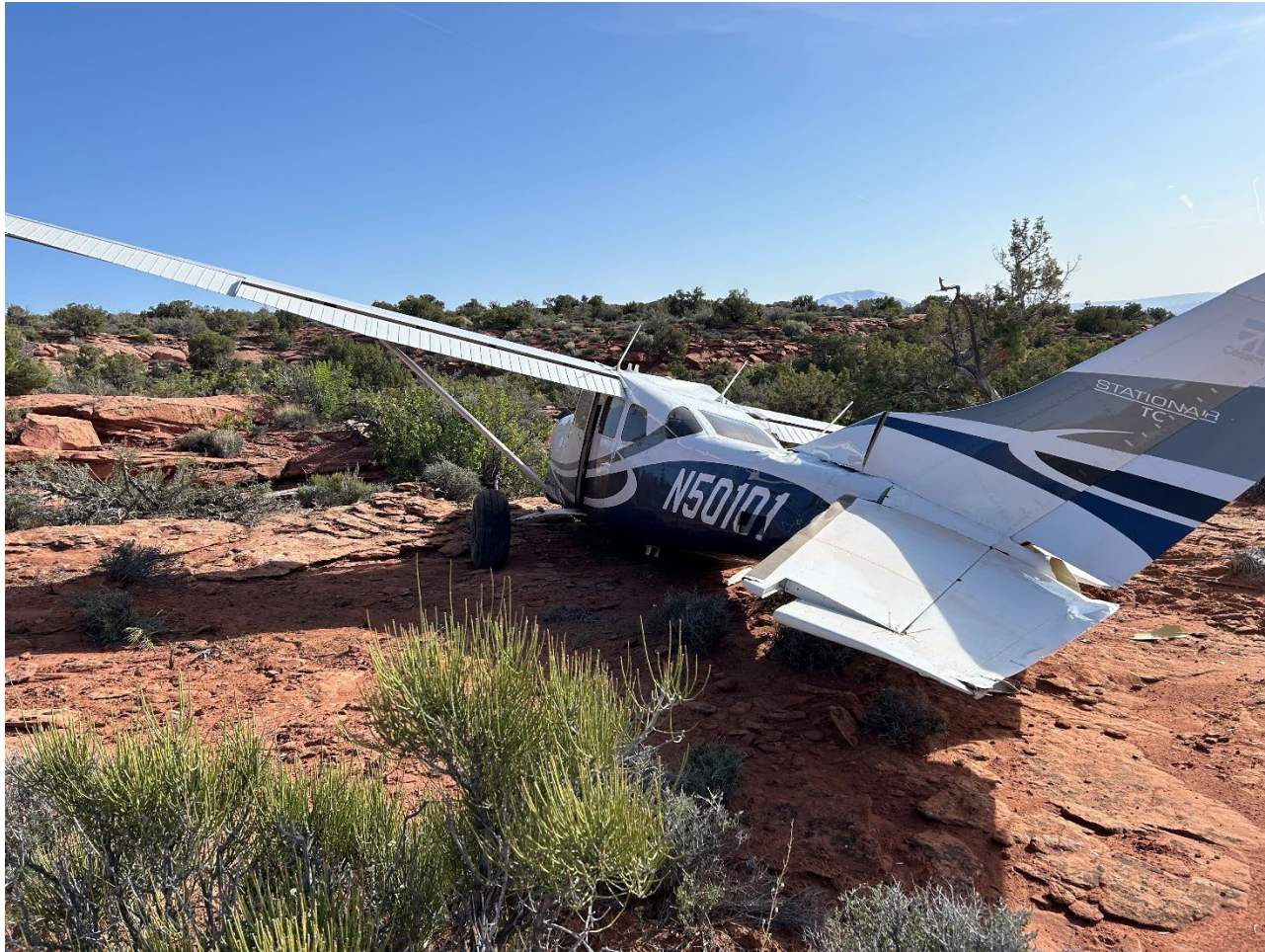
Photograph 1 - View of substantial damage to the left side empennage (Courtesy of Operator)
