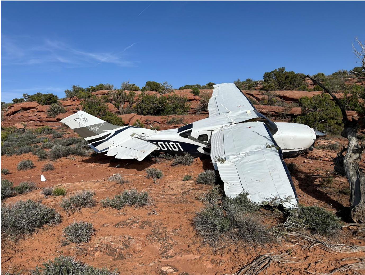
Photograph 2 - Top view of substantial damage right side empennage and right wing (Courtesy of Operator)
