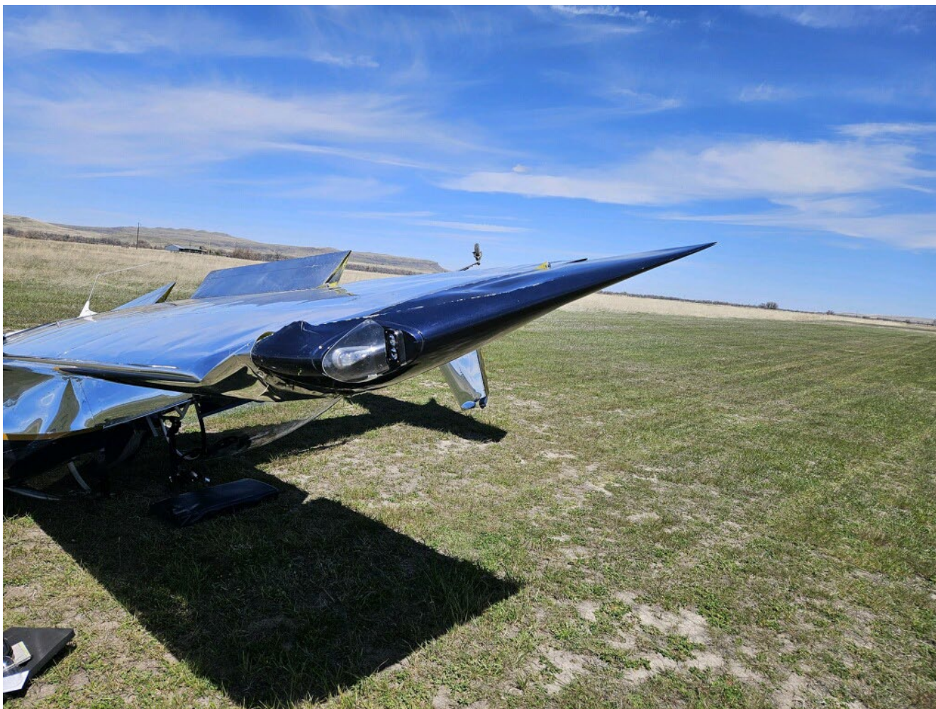
Photograph 2 - View of substantial damage to the right wing. (Courtesy of the pilot.)
