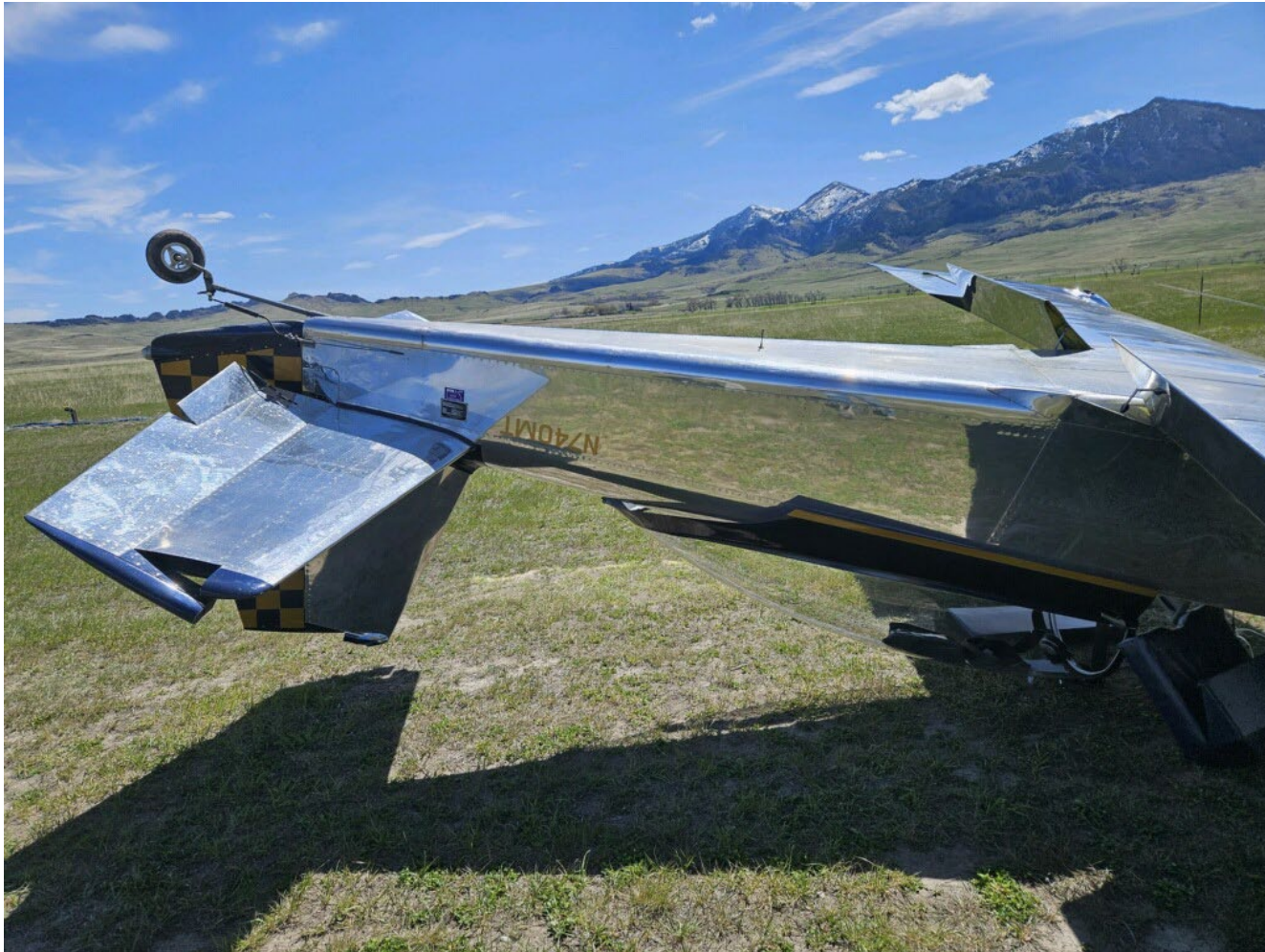
Photograph 3 - View of substantial damage to vertical stabilizer. (Courtesy of the pilot.)
